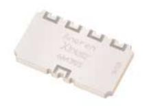
The 4A3305 is a low profile 4 way Wilkinson power divider in an easy to use surface mount package designed for DCS, PCS, UMTS, W-LAN and other 3G applications. The 4A4305 is ideal for low power, In-Phase divider/combiner applications. Parts have been run through rigorous qualification testing and units are 100% tested. They are manufactured using materials with x and y thermal expansion coefficients compatible with common substrates.
