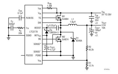
Figure 1. High Efficiency Step-Down Converter
