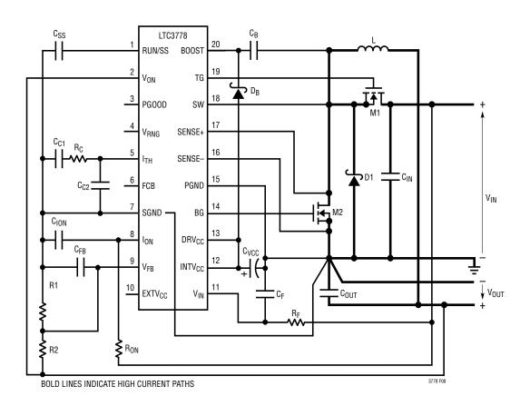
Figure 8. LTC3778 Layout Diagram
