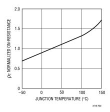
Figure 2. R<sub>DS(ON)</sub> vs. Temperature
