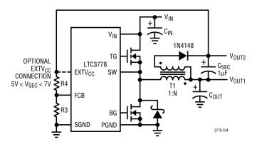
Figure 4. Secondary Output Loop and EXTV<sub>CC</sub> Connection
