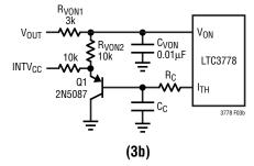
Figure 3. Correcting Frequency Shift with Load Current Changes
