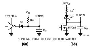
Figure 6. RUN/SS Pin Interfacing with Latchoff Defeated
