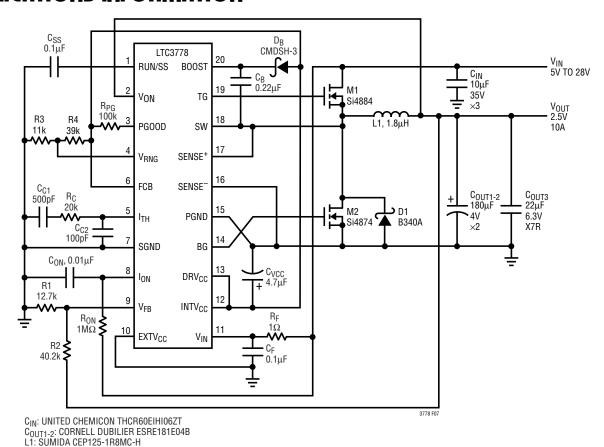
Figure 7. Design Example: 2.5V/10A at 250kHz
