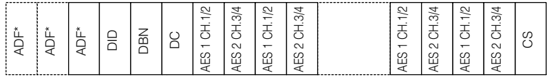
* The ancillary data flag, ADF, is one word in composite systems (ANSI/SMPTE 259M) and three words in component systems (ANSI/SMPTE 125M).
