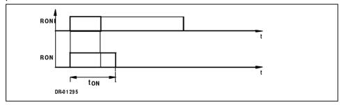
The RON output will be valid for the time that the RONI signal is high. To avoid the possibility of switching the relay to the on position for extended periods, the RON signal will stay in the on state for a maximum of 60mS, even if the RONI input is valid for a longer period.
