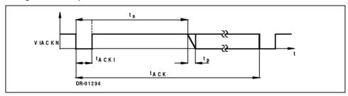
When the SA9642E device becomes operational, a watchdog acknowledge signal, from the  $\mu$ -controller must be received within a time period of  $t_{ACK}$ . If this acknowledge is not received within the time period, a reset pulse,  $t_{RES}$ , from the SA9642E is output on the RESET pin.
