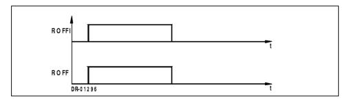
After the SA9642E has received 16 consecutive erroneous watchdog signals, the RESET pin goes low and the ROFF output display's an active high pulse for 54.9ms, every 2287.5ms period.
