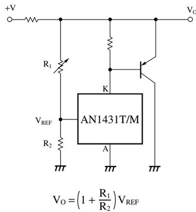
5. Adjustable output regulator combined with 3-pin regulator
