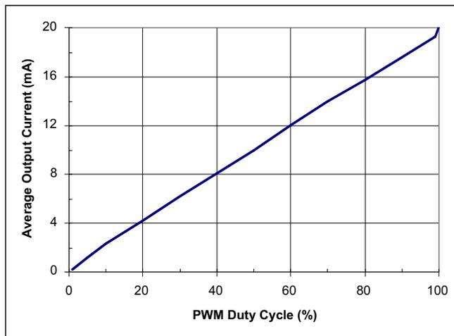
Fig. 2 Average  $I_o$  vs SHDN duty cycle
