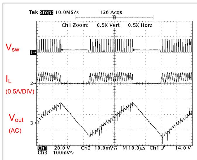
Fig. 3 Typical Switching Waveform ( $V_{in}=3.3V$ )
