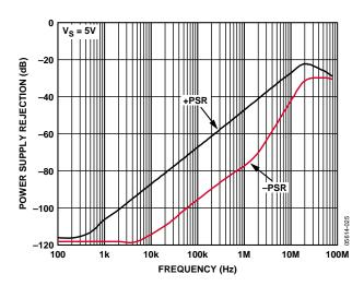
Figure 32. PSRR vs. Frequency
