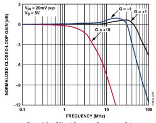
Figure 6. Small Signal Frequency Response vs. Gain
