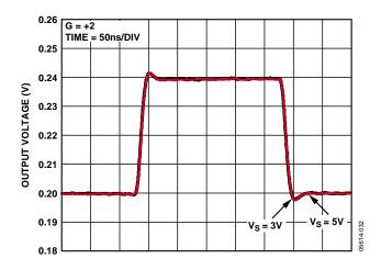
Figure 21. Small Signal Transient Response for Various Supplies
