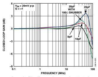
Figure 5. Small Signal Frequency Response vs. Capacitive Load
