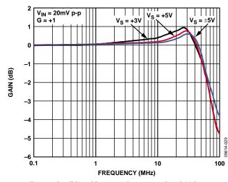
Figure 8. Small Signal Frequency Response vs. Supply Voltage
