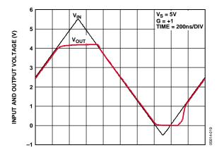
Figure 22. Input Overdrive Recovery
