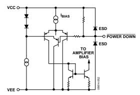
Figure 46. Power-Down Circuit
