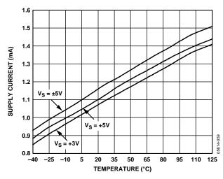
Figure 36. Supply Current vs. Temperature for Various Supplies
