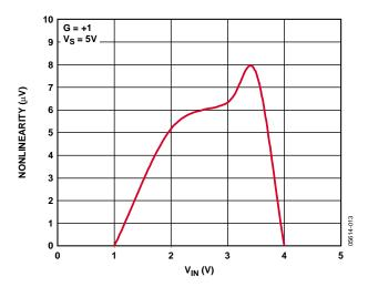
Figure 17. Nonlinearity vs. V<sub>IN</sub>
