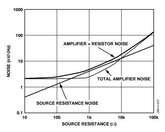
Figure 39. RTI Noise vs. Source Resistance
