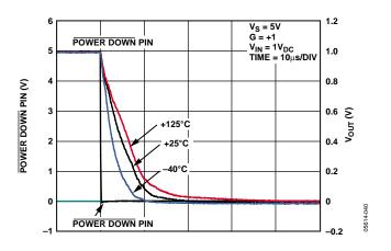
Figure 29. Power-Down Time vs. Temperature
