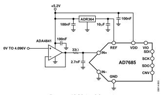
Figure 47. ADC Driver Schematic
