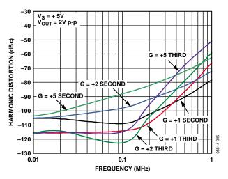
Figure 11. Harmonic Distortion vs. Frequency for Various Gains
