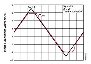
Figure 23. Output Overdrive Recovery
