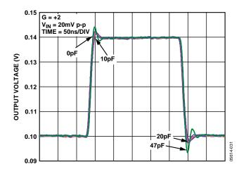
Figure 20. Small Signal Transient Response for Various Capacitive Loads
