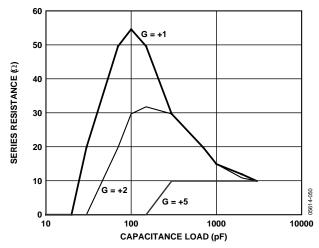
Figure 44. Series Resistance vs. Capacitive Load
