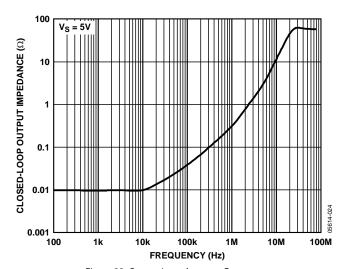
Figure 33. Output Impedance vs. Frequency
