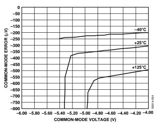
Figure 41. Vos vs. -CMP vs. Common-Mode Error
