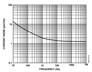
Figure 15. Current Noise vs. Frequency
