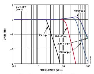
Figure 9. Frequency Response for Various  $V_{\text{OUT}}$
