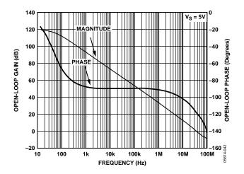
Figure 10. Open-Loop Gain and Phase vs. Frequency
