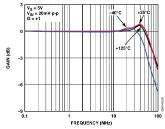
Figure 7. Small Signal Frequency Response vs. Temperature
