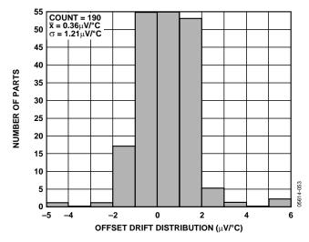
Figure 16. Input Offset Voltage Distribution
