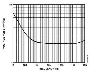
Figure 14. Voltage Noise vs. Frequency
