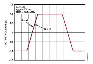
Figure 24. Large Signal Transient Response for Various Gains
