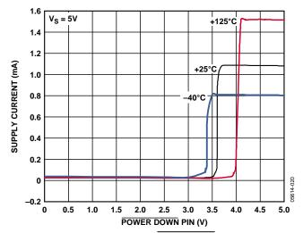
Figure 30. Supply Current vs. POWER DOWN Pin Voltage
