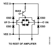
Figure 45. Input Stage and Protection Diodes
