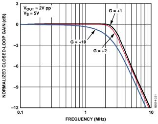
Figure 4. Large Signal Frequency Response vs. Gain
