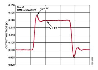
Figure 25. Small Signal Transient Response for Various Supplies
