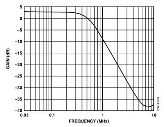
Figure 49. Filter Frequency Response
