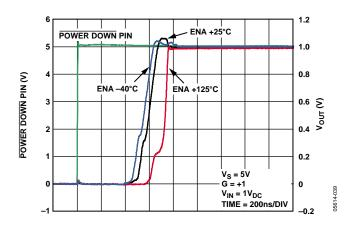
Figure 28. Power-Up Time vs. Temperature
