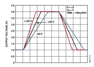
Figure 26. Output Voltage vs. Temperature
