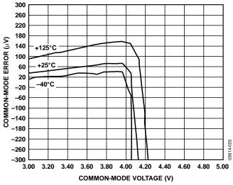
Figure 40. Vos vs. +CMP vs. Common-Mode Error
