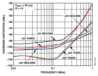
Figure 13. Harmonic Distortion vs. Frequency for Various Supplies
