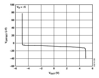
Figure 18. Input Error Voltage vs. Output Voltage
