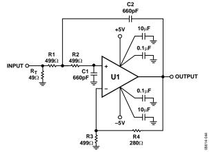
Figure 48. Two-Pole 500 kHz Reconstruction Filter Schematic
