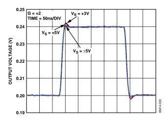
Figure 19. Small Signal Transient Response for Various Supplies
