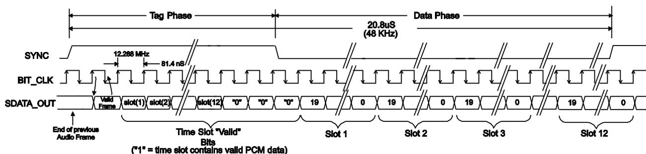
Figure 31. AC-Link Audio Output Frame
