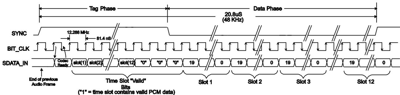
Figure 33. AC-Link Audio Input Frame
