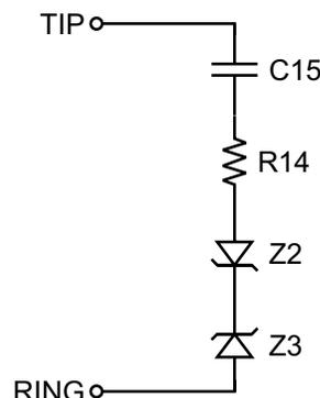
Figure 24. Ringer Impedance Network
