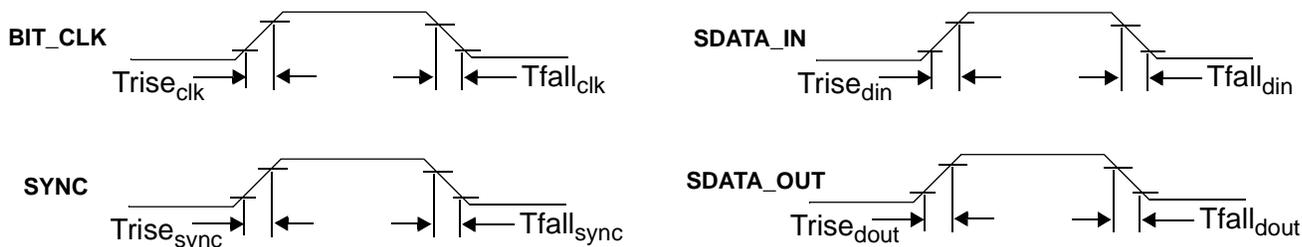
**Figure 6. Signal Rise and Fall Timing Diagram**
