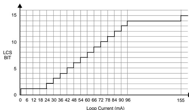
**Figure 28. Typical LCS Transfer Function**
