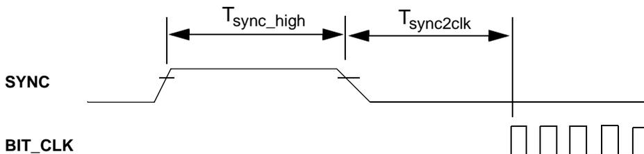
**Figure 3. Warm Reset Timing Diagram**
