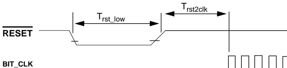
**Figure 2. Cold Reset Timing Diagram**
