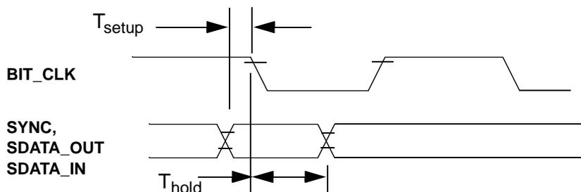
**Figure 5. Data Setup and Hold Timing Diagram**
