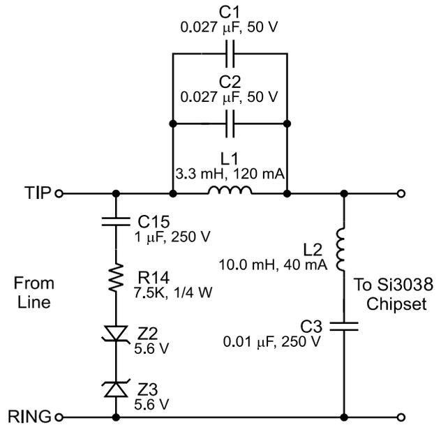
Figure 27. Dongle Applications Circuit
