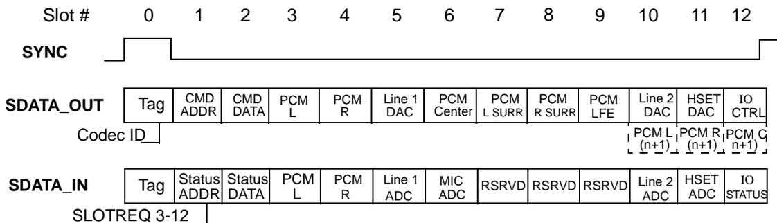
**Figure 30. Standard Bi-Directional Audio Frame**
