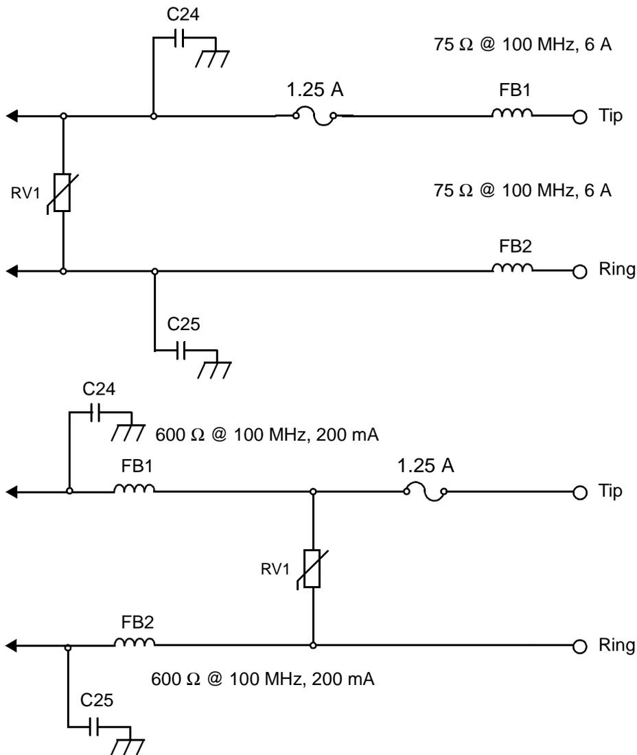
**Figure 36. Circuits that Pass all UL1950 Overvoltage Tests**
