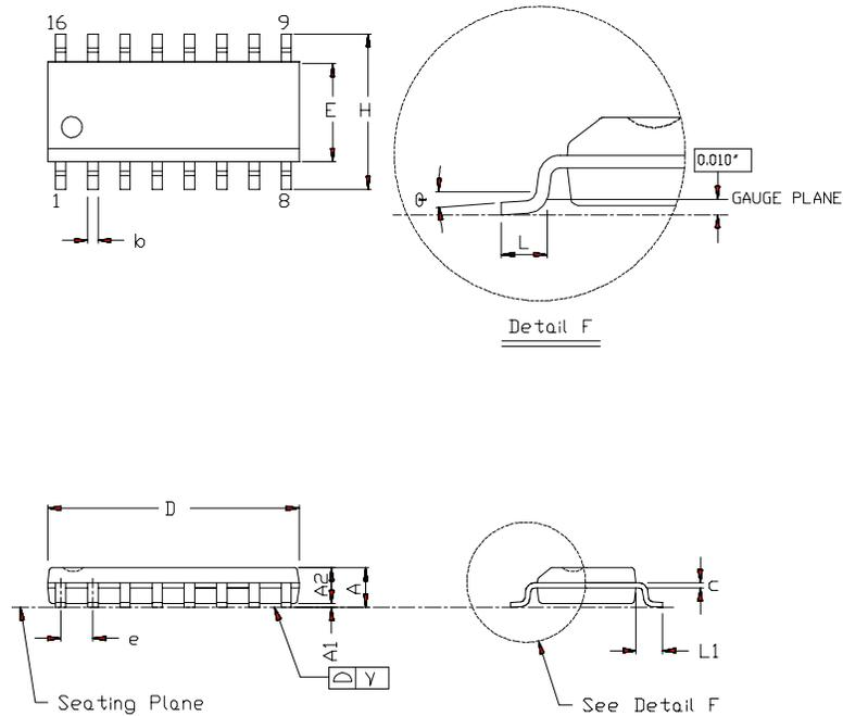
**Figure 38. 16-pin Small Outline Plastic Package (SOIC)**
