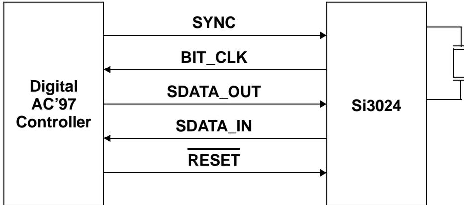
**Figure 29. Si3038 Connection To AC'97 Controller (Primary Device Configuration)**
