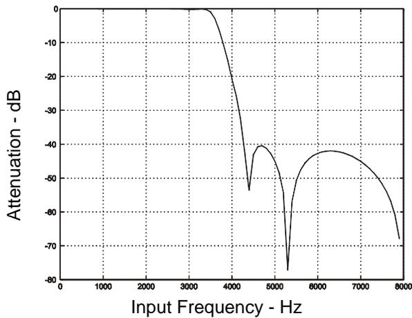
**Figure 13. IIR Receive Filter Response**
