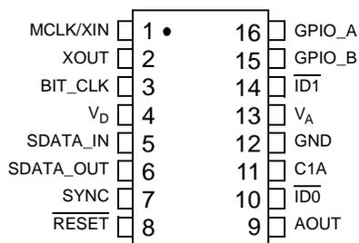
Figure 37. Si3024 Pin Configuration
