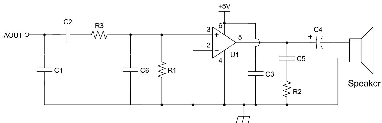
Figure 20. Optional Connection to AOUT for a Call Progress Speaker
