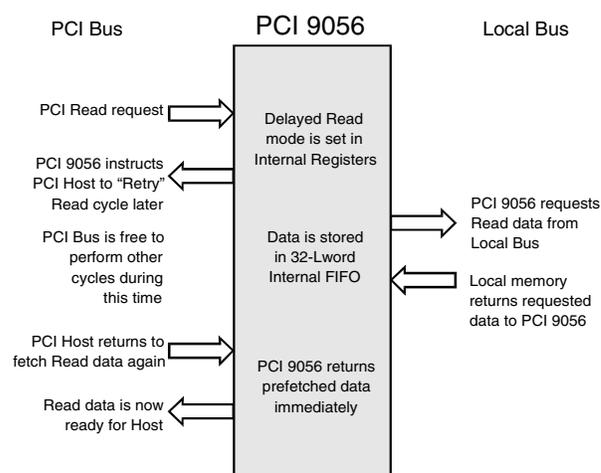
Figure 5-6. Direct Slave Delayed Read
