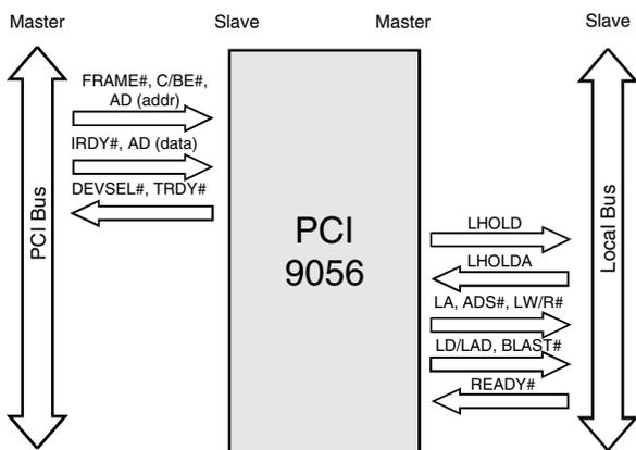
Figure 5-8. Direct Slave Write
