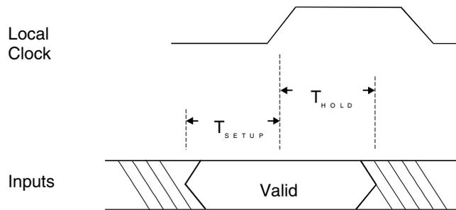
Figure 13-1. PCI 9056 Local Input Setup and Hold Waveform
