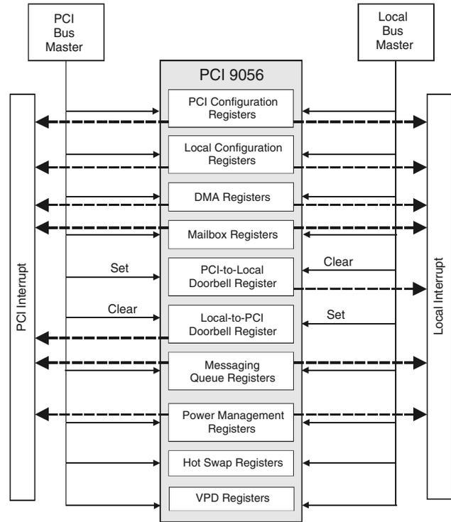
**Figure 2-6. PCI 9056 Internal Register Access**
