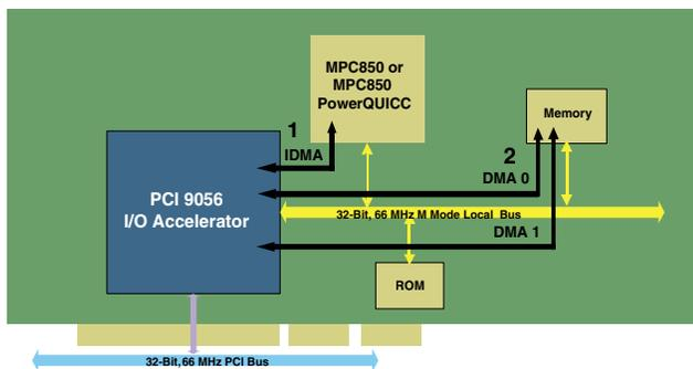
**Figure 1-3. High-Performance MPC850 or MPC860 PowerQUICC Adapter Design**
