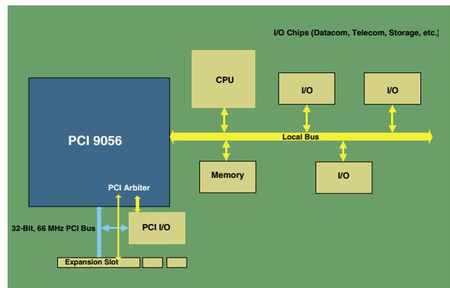
**Figure 1-8. PCI 9056 Embedded Host System with Generic Host CPU**
