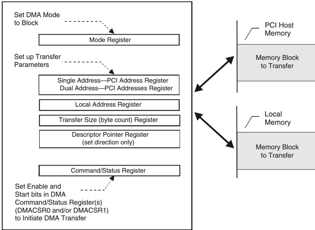
Figure 5-11. Block DMA Mode Initialization (Single Address or Dual Address PCI)
