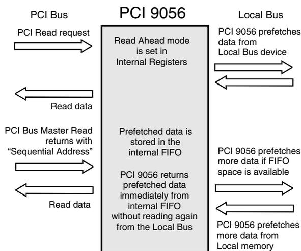
Figure 3-7. Direct Slave Read Ahead Mode
