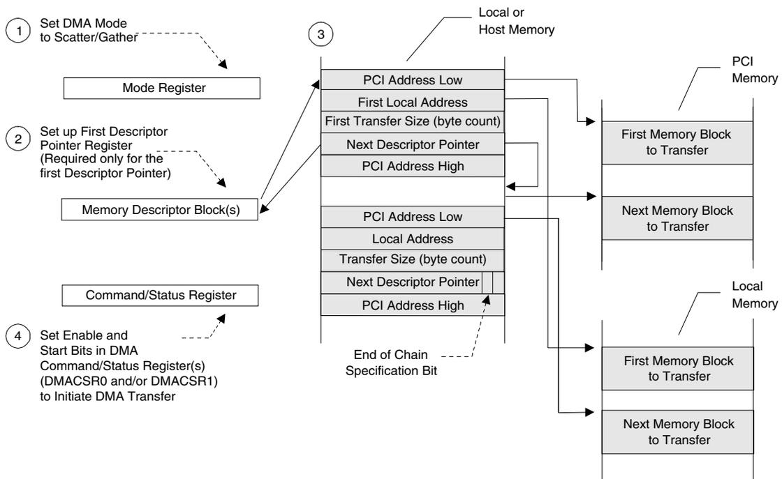
Figure 3-18. Scatter/Gather DMA Mode Descriptor Initialization [DAC PCI Address (DMAMODE0[18] and/or DMAMODE1[18]) Descriptor Dependent (PCI Address High Added)]
