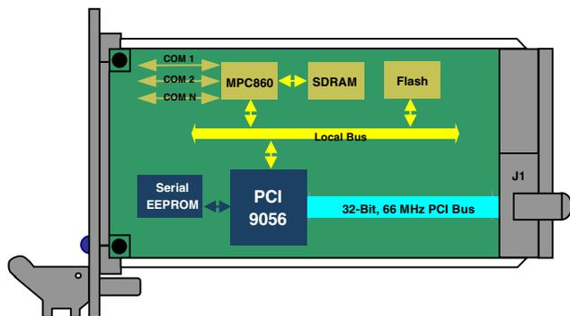
Figure 1-4. PCI 9056 CompactPCI Peripheral Card
