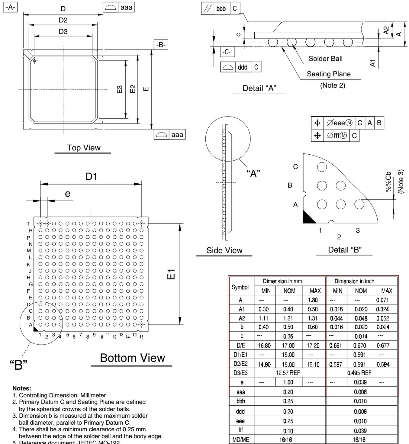
Figure 14-1. Mechanical Dimensions—Top, Side, and Bottom Views
