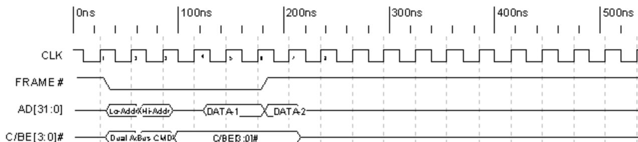
Figure 3-14. Dual Address Timing
