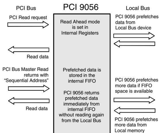
Figure 5-7. Direct Slave Read Ahead Mode
