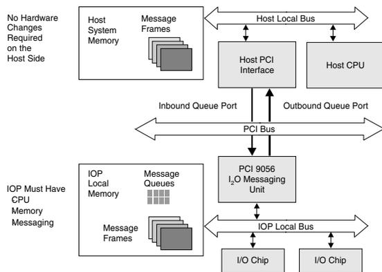
**Figure 7-1. Typical I<sub>2</sub>O Server/Adapter Card Design**
