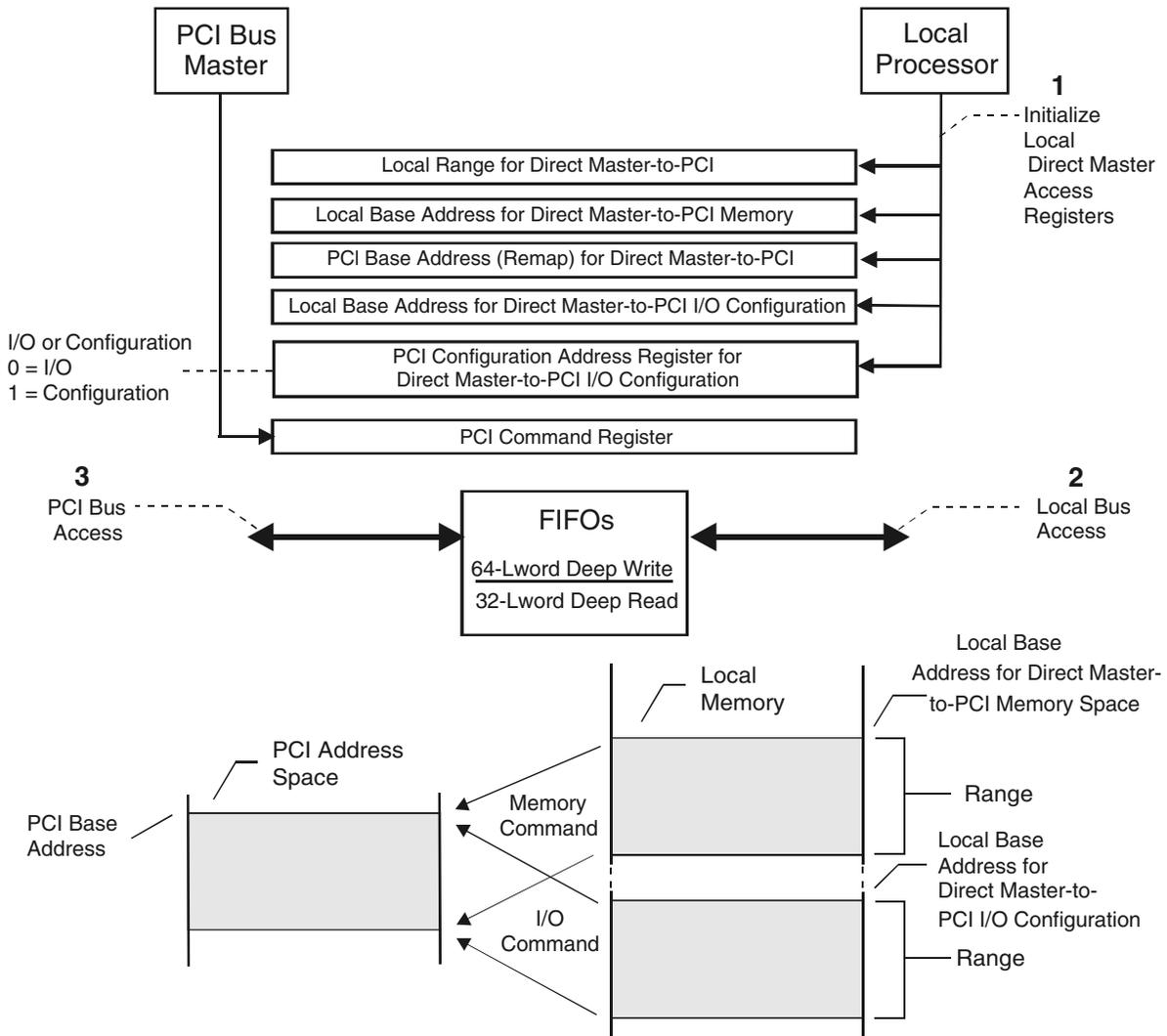
Figure 3-1. Direct Master Access to the PCI Bus
