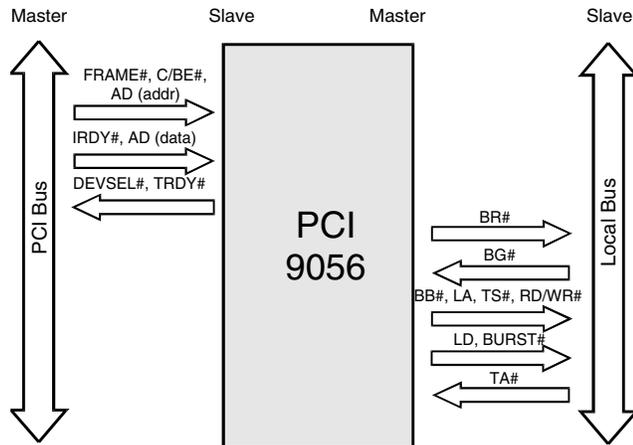
Figure 3-8. Direct Slave Write
