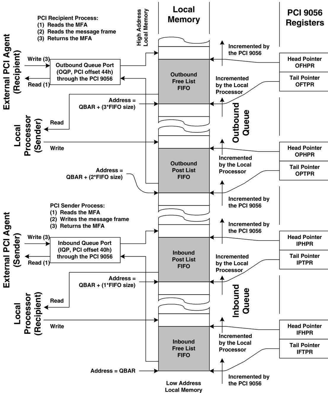
Figure 7-3. I<sub>2</sub>O Circular FIFO Operation
