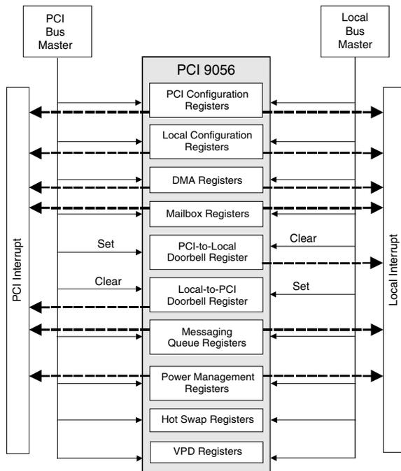
Figure 4-6. PCI 9056 Internal Register Access
