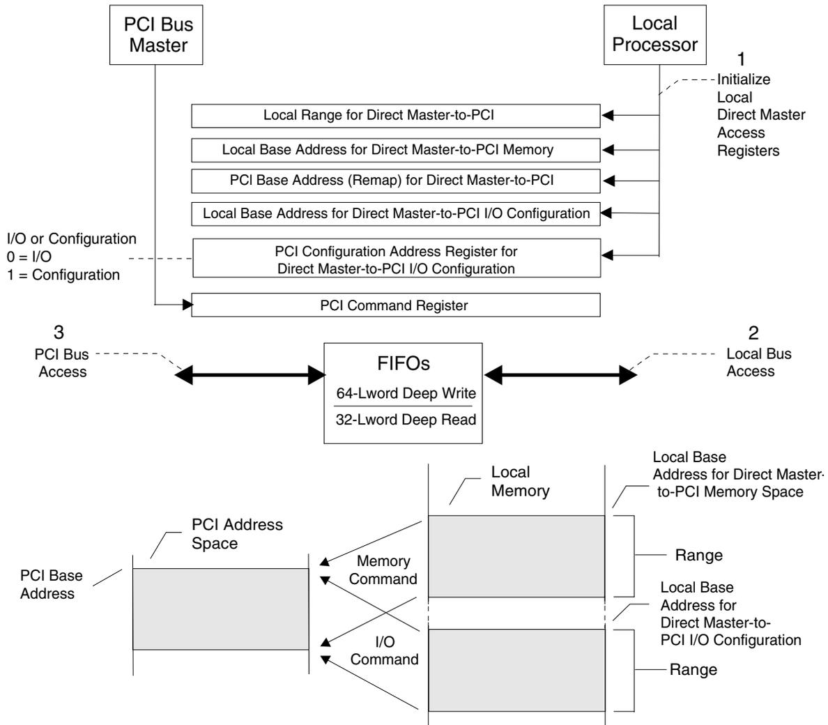
Figure 5-1. Direct Master Access of the PCI Bus
