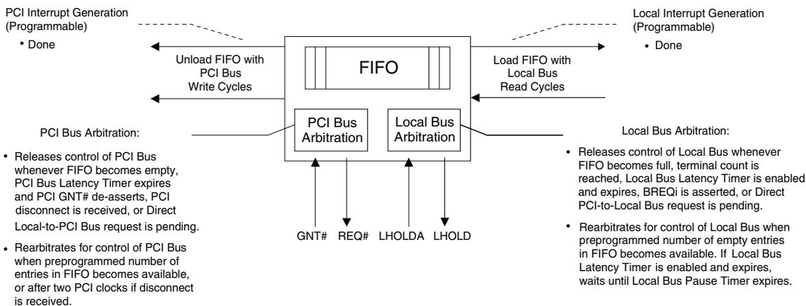
Figure 5-19. Local-to-PCI Bus DMA Data Transfer Operation
