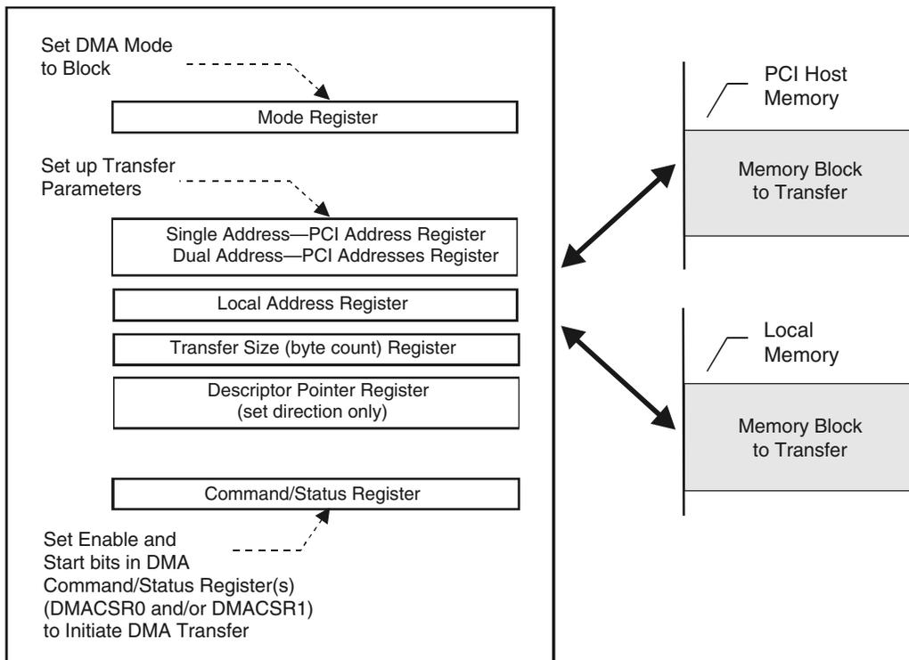
Figure 3-11. Block DMA Mode Initialization (Single Address or Dual Address PCI)
