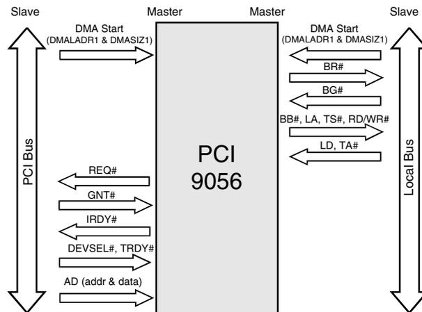
Figure 3-13. DMA, Local-to-PCI Bus
