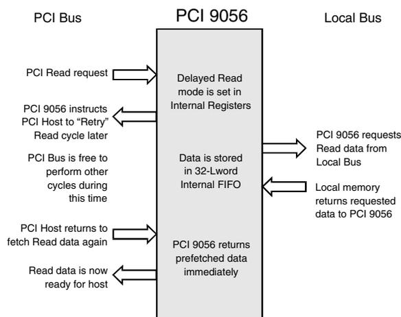
Figure 3-6. Direct Slave Delayed Read
