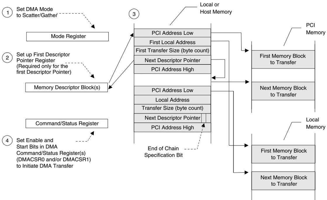
Figure 5-18. Scatter/Gather DMA Mode Descriptor Initialization [DAC PCI Address (DMAMODE0[18] and/or DMAMODE1[18]) Descriptor Dependent] (PCI Address High Added)
