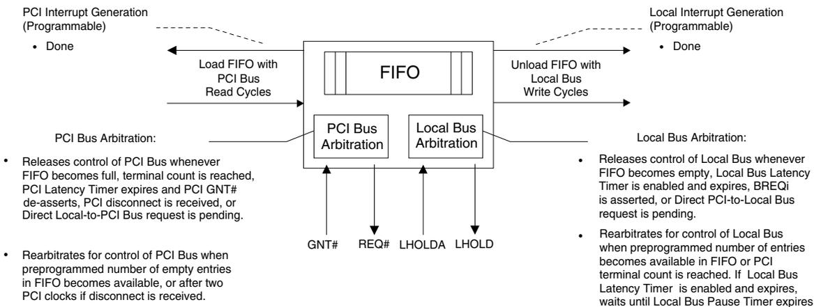
Figure 5-20. PCI-to-Local Bus DMA Data Transfer Operation
