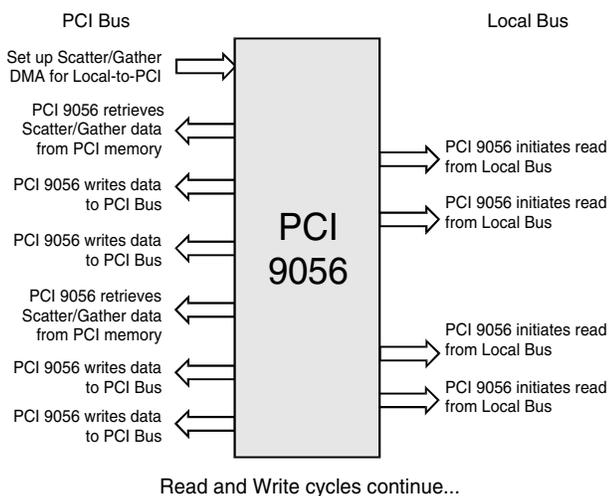
**Figure 5-16. Scatter/Gather DMA Mode from Local-to-PCI Bus (Control Access from the PCI Bus)**
