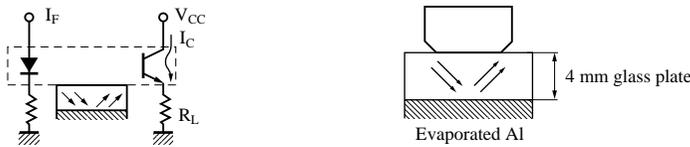
\*2 Switching time measurement circuit
