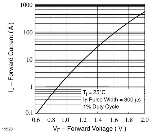
Figure 2. Typ. Forward Current vs. Forward Voltage
