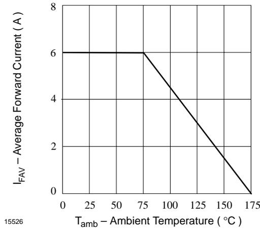
Figure 1. Max. Average Forward Current vs. Ambient Temperature
