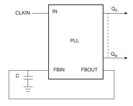
Note: Feedback capacitor value 'C' is to be determined based on the phase characteristics of the PLL.
