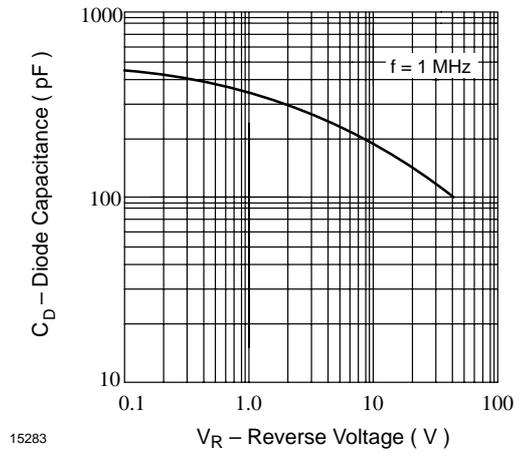
Figure 4. Typ. Diode Capacitance vs. Reverse Voltage
