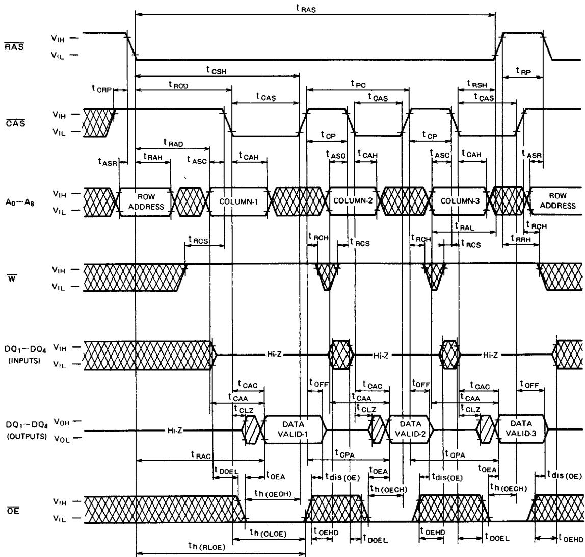
**FAST PAGE MODE 1048576-BIT(262144-WORD BY 4-BIT)DYNAMIC RAM****Fast Page Mode Write Cycle (Early Write)**
