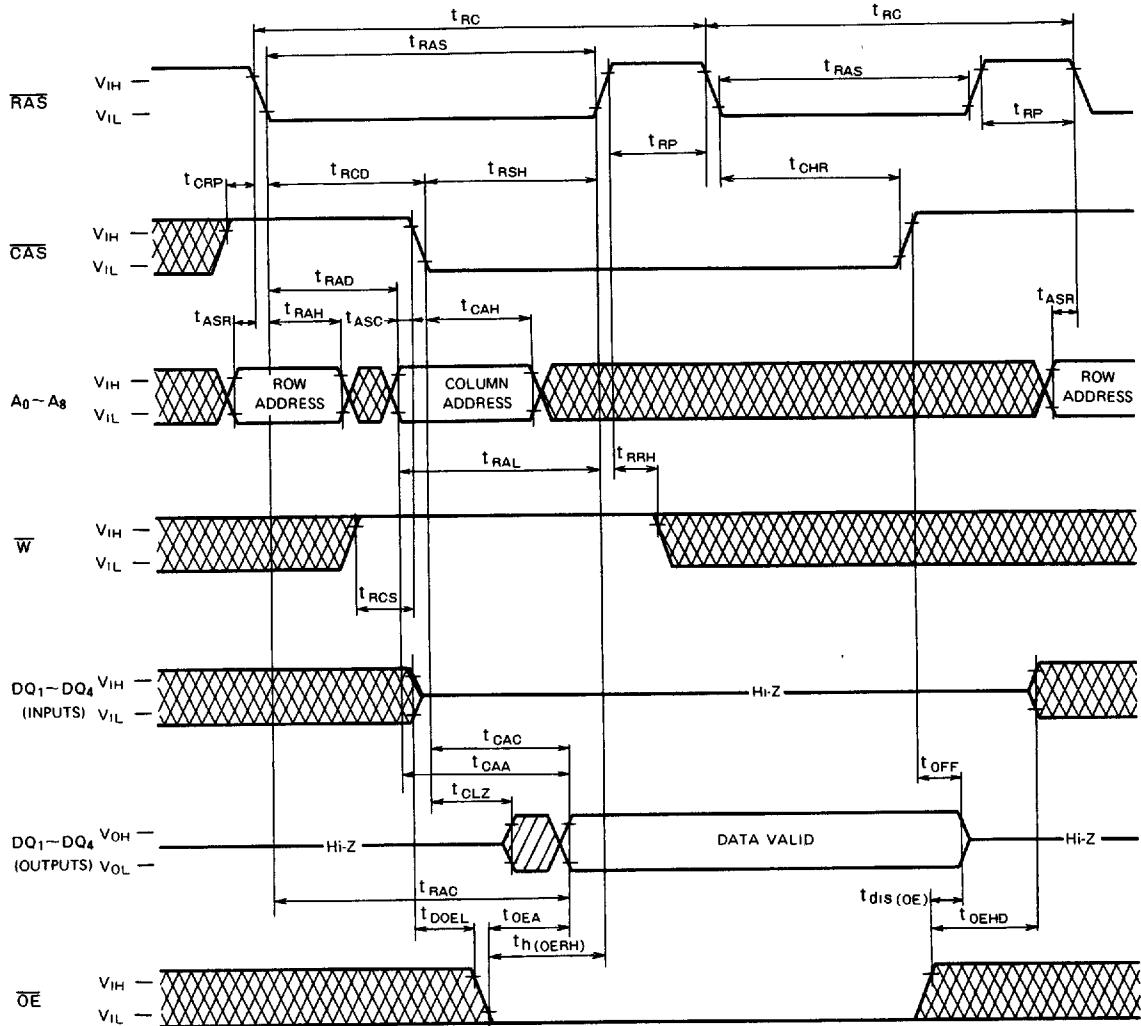
Note 26: Early write, delayed write, read-write or read-modify-write cycle is applicable instead of read cycle
