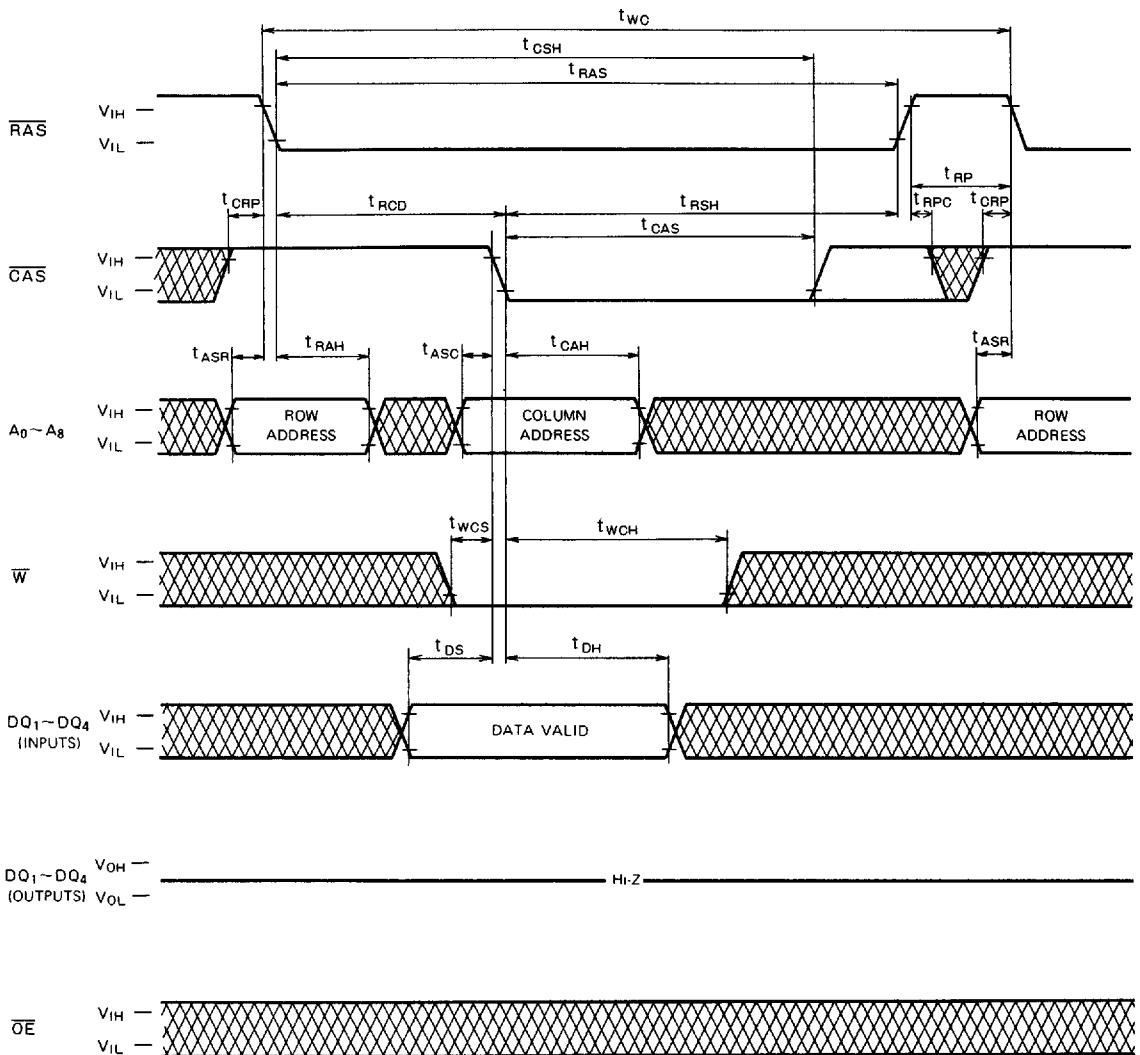
**M5M44256BP, J, L, VP, RV-7, -8, -10****FAST PAGE MODE 1048576-BIT(262144-WORD BY 4-BIT)DYNAMIC RAM****Write Cycle (Delayed Write)**
