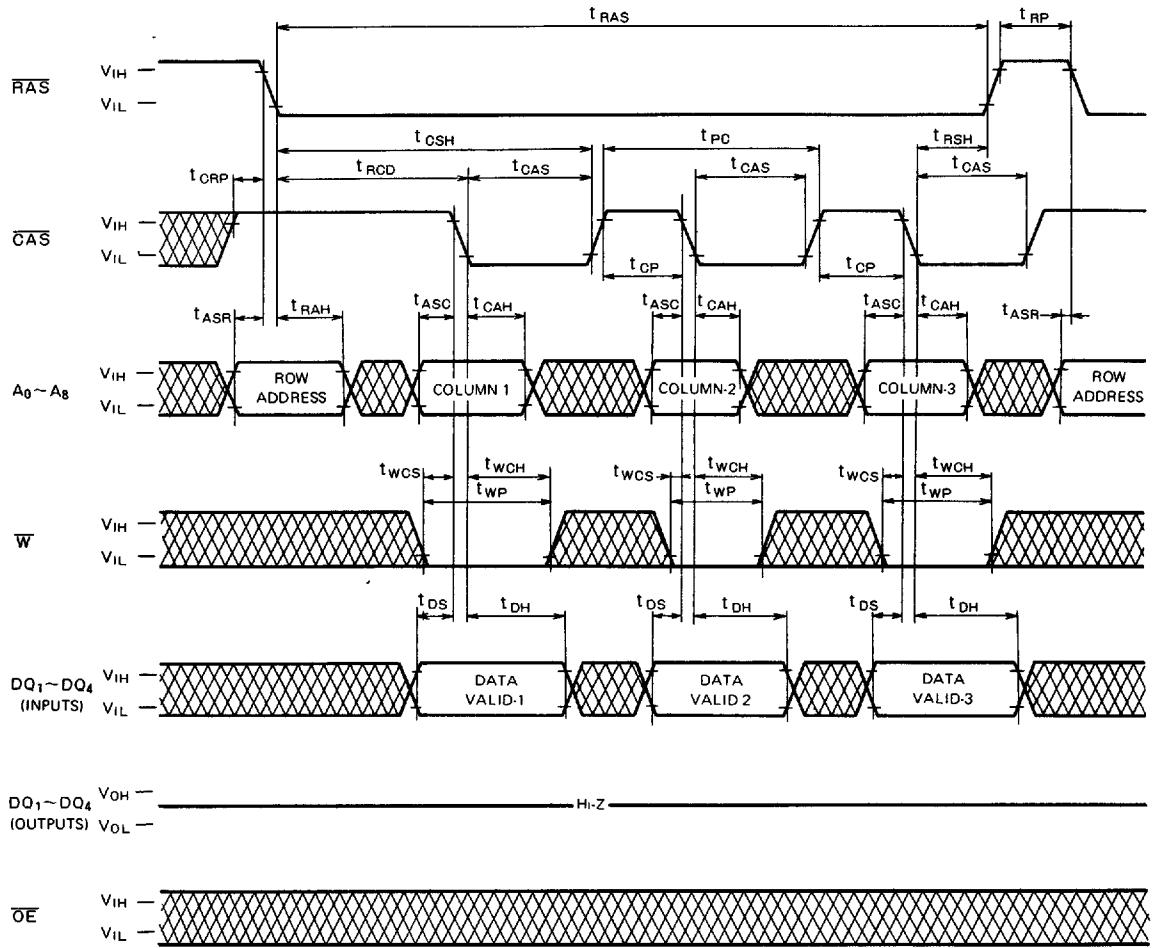
**FAST PAGE MODE 1048576-BIT(262144-WORD BY 4-BIT)DYNAMIC RAM****Fast Page Mode Write Cycle (Delayed Write)**
