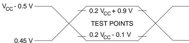
Note: 1. AC Inputs during testing are driven at  $V_{CC} - 0.5 \text{ V}$  for a logic 1 and  $0.45 \text{ V}$  for a logic 0. Timing measurements are made at  $V_{IHmin}$ . for a logic 1 and  $V_{ILmax}$ . for a logic 0.
