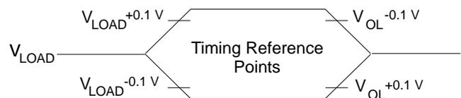
Note: 1. For timing purposes, a port pin is no longer floating when a  $100 \text{ mV}$  change from load voltage occurs. A port pin begins to float when a  $100 \text{ mV}$  change from the loaded  $V_{OH}/V_{OL}$  level occurs.
