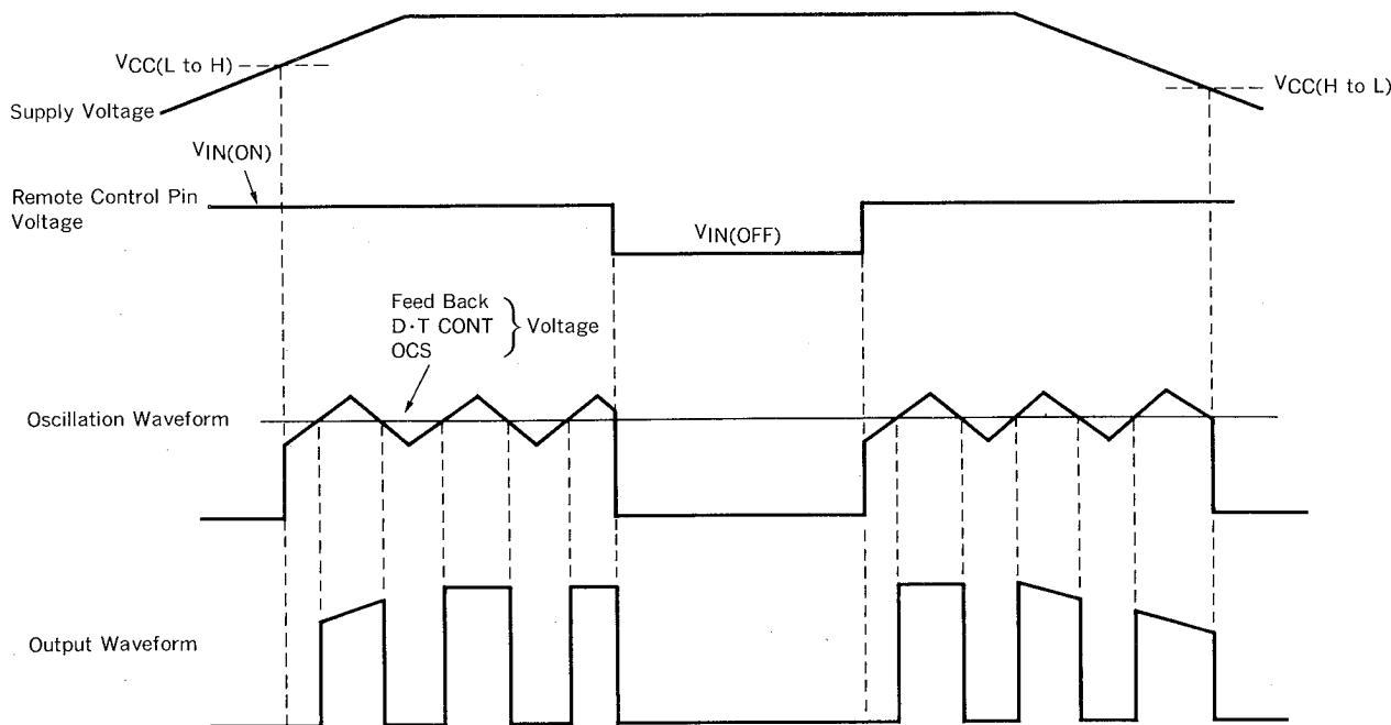
ELECTRICAL CHARACTERISTICS ( $T_a = 25^\circ\text{C}$ ,  $V_{CC} = 15 \text{ V}$ ,  $R_T = 36 \text{ k}\Omega$ ,  $C_T = 1 \text{ 000 pF}$ ,  $f_{osc} = 200 \text{ kHz}$ )
