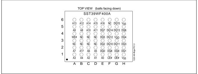
FIGURE 1: PIN ASSIGNMENTS FOR 48-BALL TFBGA
