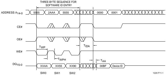
Note: Device ID = 272FH for SST39WF400A X can be  $V_{IL}$  or  $V_{IH}$ , but no other value.
