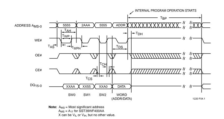
FIGURE 4: WE# CONTROLLED PROGRAM CYCLE TIMING DIAGRAM
