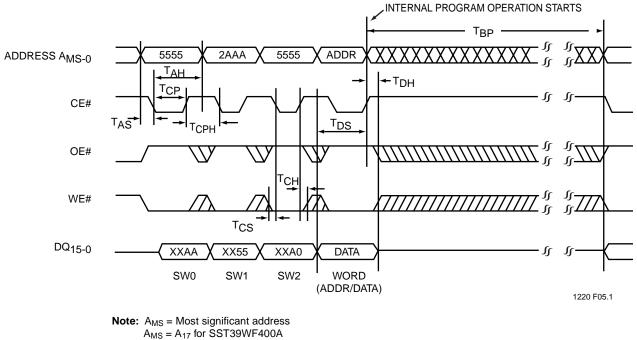
$A_{MS} = A_{17}$  for SST39WF400A X can be V<sub>IL</sub> or V<sub>IH</sub>, but no other value.
