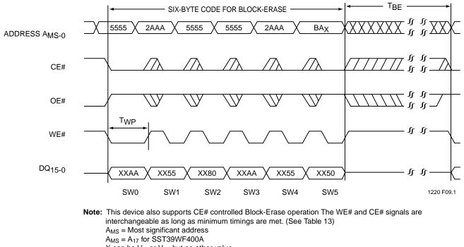
X can be  $V_{IL}$  or  $V_{IH}$ , but no other value.
