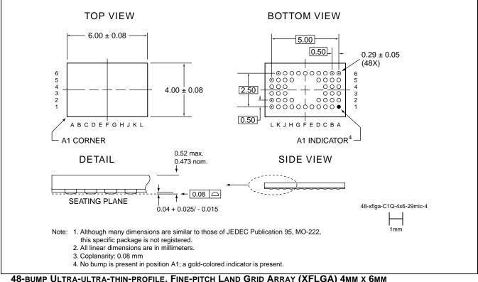
48-BUMP ULTRA-ULTRA-THIN-PROFILE, FINE-PITCH LAND GRID ARRAY (XFLGA) 4MM X 6MM SST PACKAGE CODE: C1Q
