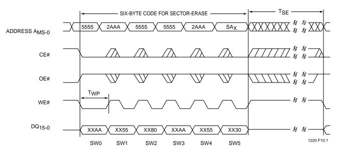
**Note:** This device also supports CE# controlled Sector-Erase operation The WE# and CE# signals are interchangeable as long as minimum timings are met. (See Table 13)
