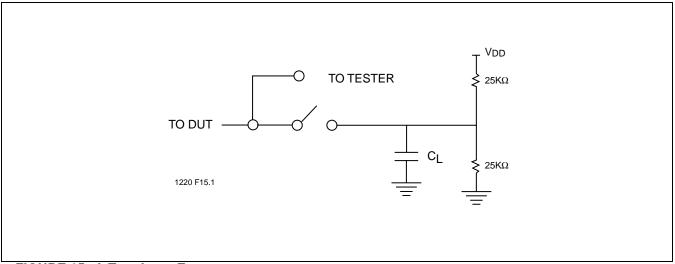
FIGURE 15: A TEST LOAD EXAMPLE
