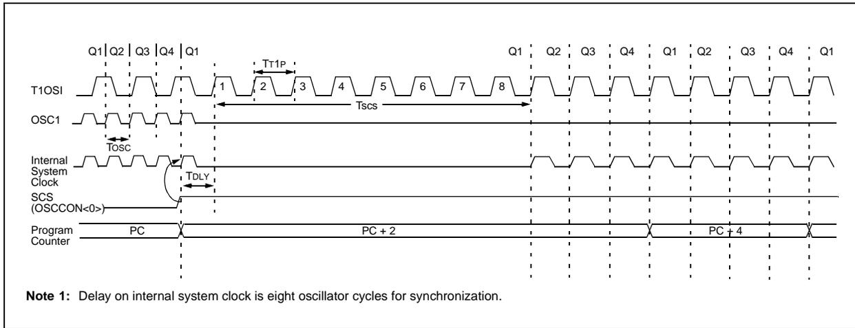
The sequence of events that takes place when switching from the Timer1 oscillator to the main oscillator will depend on the mode of the main oscillator. In addition to eight clock cycles of the main oscillator, additional delays may take place.
