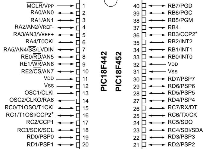
**Note:** Pin compatible with 40-pin PIC16C7X devices.
