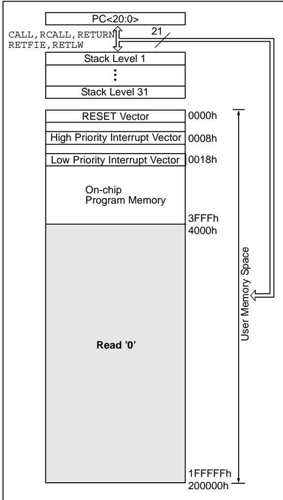
**FIGURE 4-2: PROGRAM MEMORY MAP AND STACK FOR PIC18F452/252**
