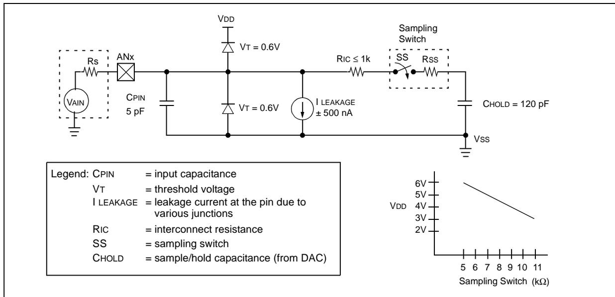
To calculate the minimum acquisition time, Equation 17-1 may be used. This equation assumes that 1/2 LSB error is used (1024 steps for the A/D). The 1/2 LSB error is the maximum error allowed for the A/D to meet its specified resolution.
