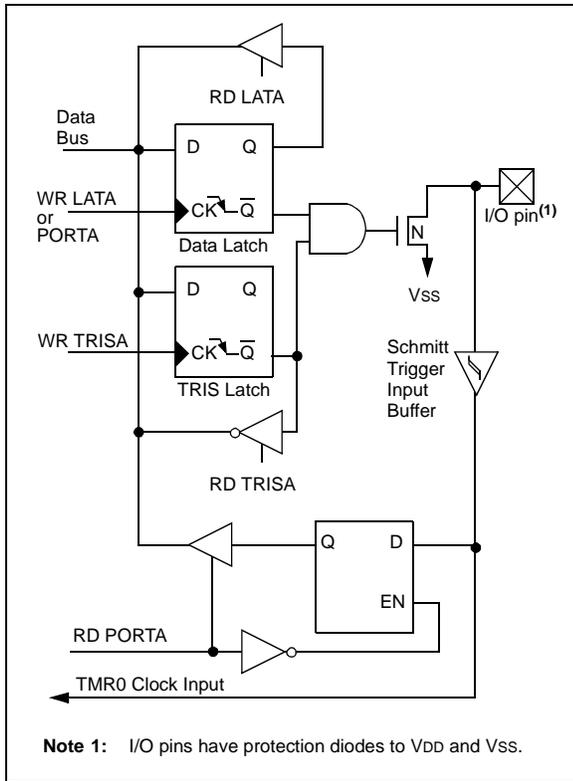
**FIGURE 9-3: BLOCK DIAGRAM OF RA6**
