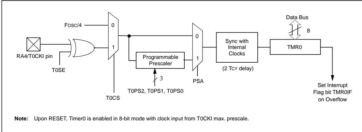
**FIGURE 10-2: TIMER0 BLOCK DIAGRAM IN 16-BIT MODE**
