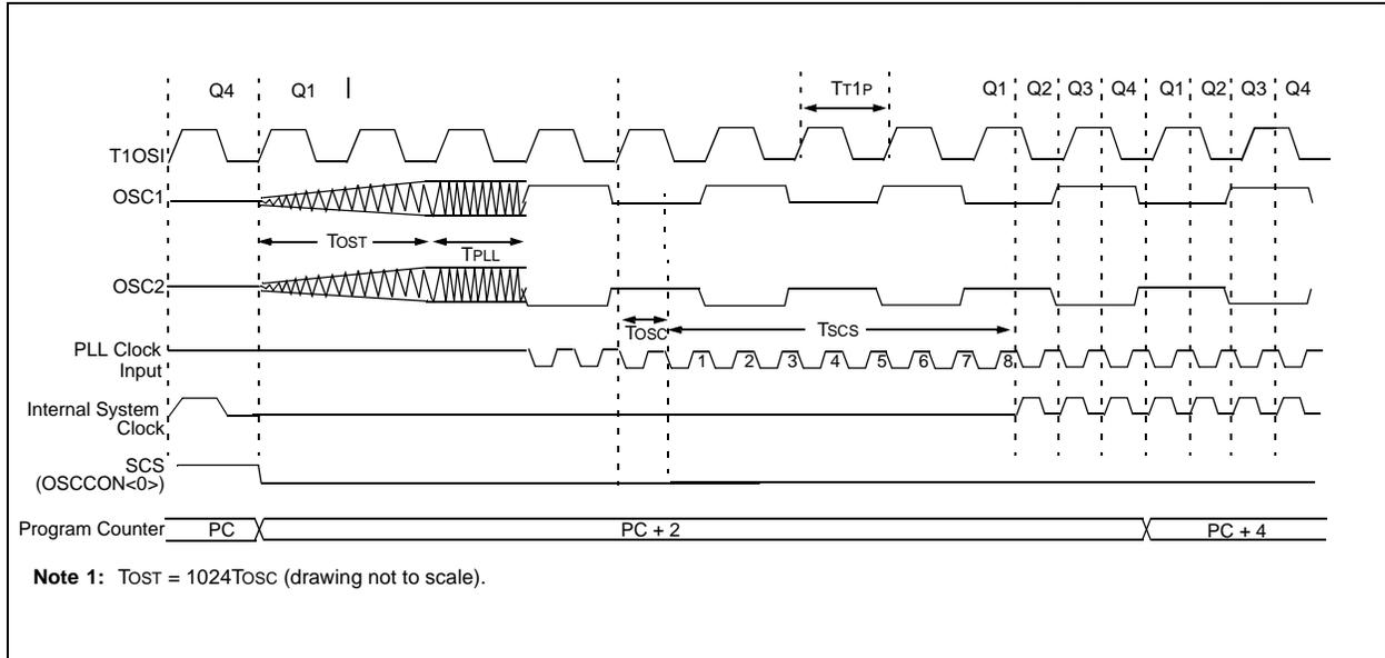
If the main oscillator is configured in the RC, RCIO, EC or ECIO modes, there is no oscillator start-up time-out. Operation will resume after eight cycles of the main oscillator have been counted. A timing diagram, indicating the transition from the Timer1 oscillator to the main oscillator for RC, RCIO, EC and ECIO modes, is shown in Figure 2-11.
