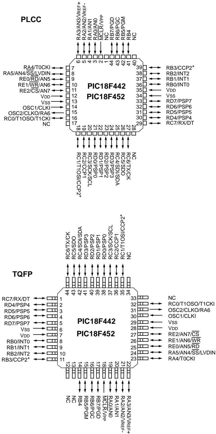
\* RB3 is the alternate pin for the CCP2 pin multiplexing.
