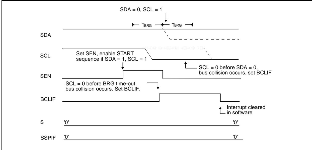
**FIGURE 15-28: BRG RESET DUE TO SDA ARBITRATION DURING START CONDITION**
