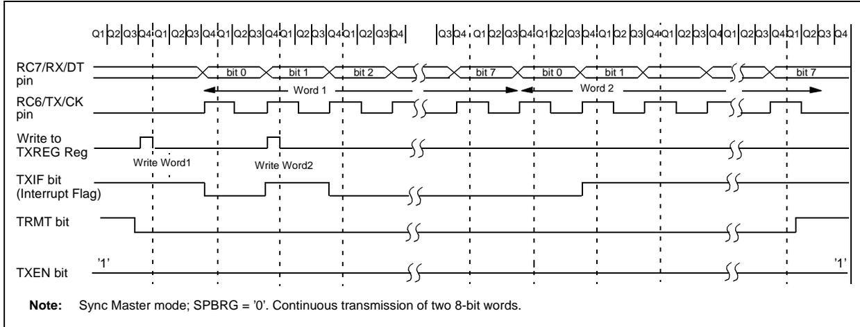
**FIGURE 16-7: SYNCHRONOUS TRANSMISSION (THROUGH TXEN)**
