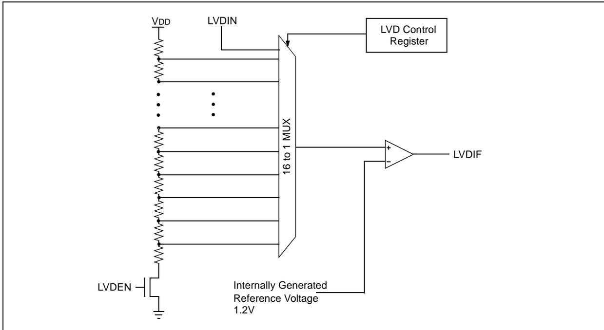
The LVD module has an additional feature that allows the user to supply the trip voltage to the module from an external source. This mode is enabled when bits LVDL3:LVDL0 are set to 1111. In this state, the comparator input is multiplexed from the external input pin,
