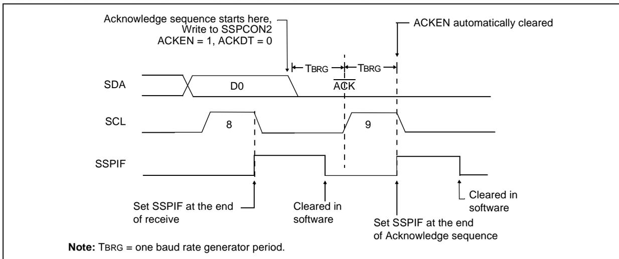
**FIGURE 15-24: STOP CONDITION RECEIVE OR TRANSMIT MODE**
