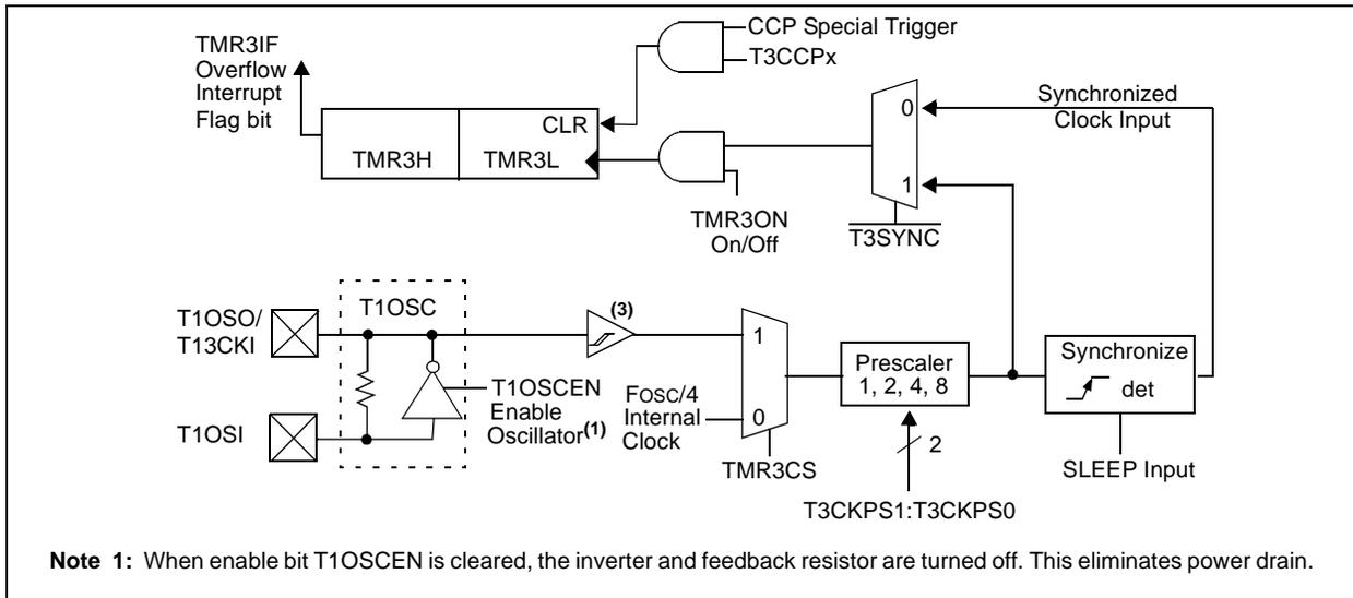
**FIGURE 13-2: TIMER3 BLOCK DIAGRAM CONFIGURED IN 16-BIT READ/WRITE MODE**
