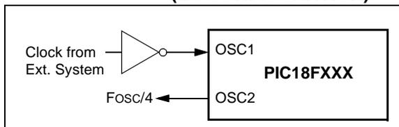
The ECIO oscillator mode functions like the EC mode, except that the OSC2 pin becomes an additional general purpose I/O pin. The I/O pin becomes bit 6 of PORTA (RA6). Figure 2-5 shows the pin connections for the ECIO oscillator mode.
