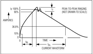
Figure 5b. Human Body Model Current Waveform
