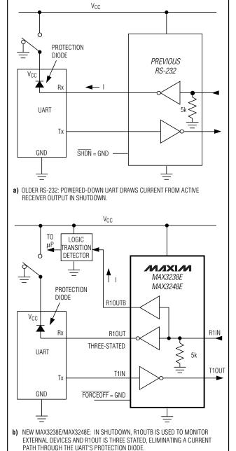
Figure 2. MAX3238E/MAX3248E detect RS-232 activity when the UART and interface are shut down.
