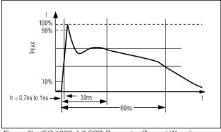
Figure 6b. IEC 1000-4-2 ESD Generator Current Waveform
