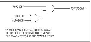
Figure 3d. Power-Down Logic
