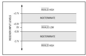
Figure 4a. Receiver Positive/Negative Thresholds for INVALID
