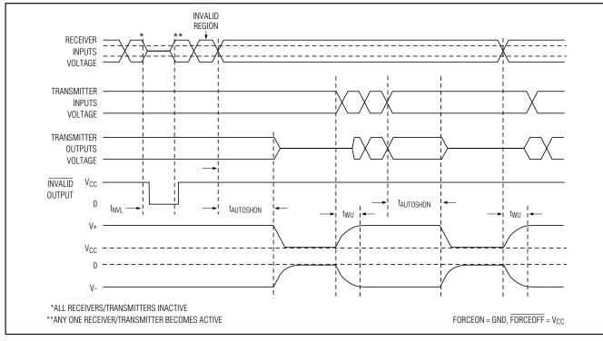
Figure 4b. AutoShutdown Plus and INVALID Timing Diagram
