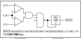
Figure 3b. INVALID Functional Diagram, INVALID High
