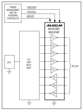
Figure 1. Interface Under Control of PMU
