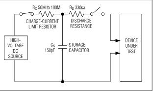
Figure 6a. IEC 1000-4-2 ESD Test Model
