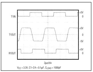
Figure 10. Loopback Test Result at 250kbps
