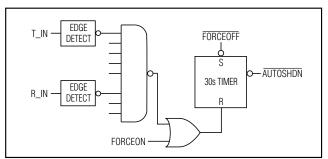
Figure 3c. AutoShutdown Plus Logic
