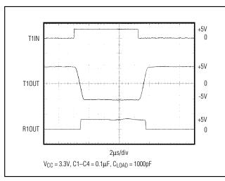
Figure 9. Loopback Test Result at 120kbps
