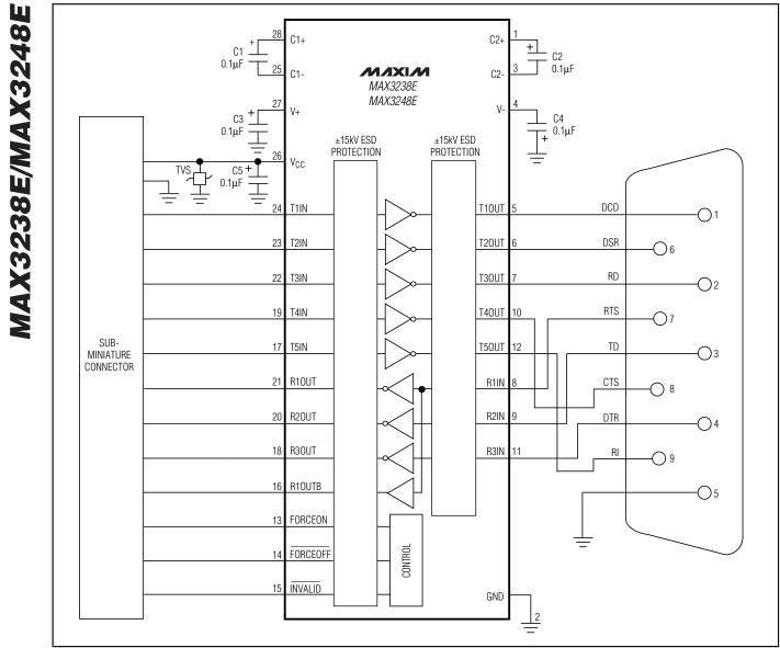
Figure 11. Data Cable Application Example
