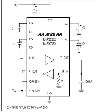
Figure 8. Loopback Test Circuit
