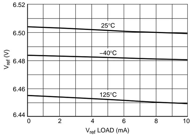
Figure 21. V<sub>ref</sub> Load Regulation
