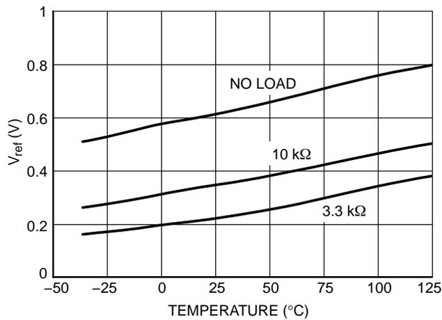
Figure 22. V<sub>ref</sub> in Shutdown Condition
