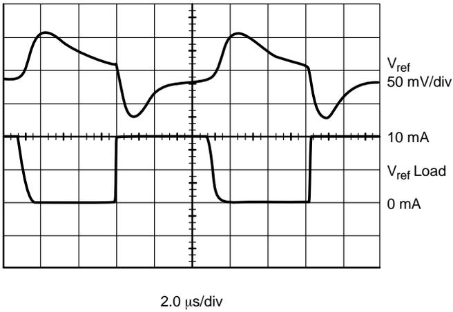
**Figure 18. Transient Response for 6.5 Volt Reference**
