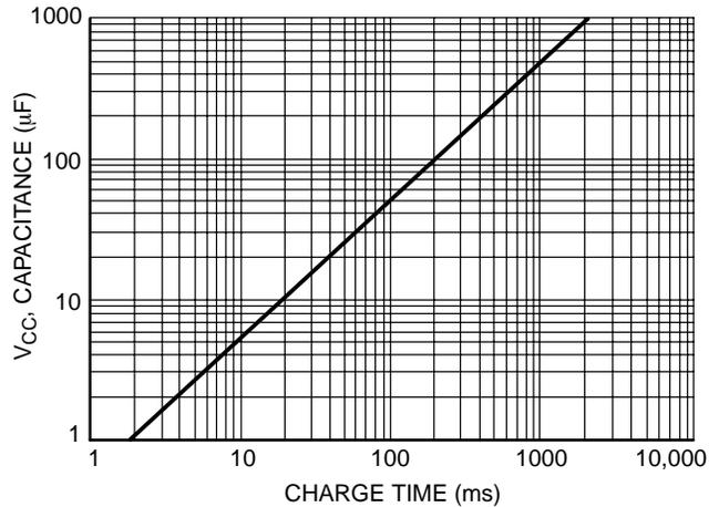
Figure 13. V<sub>CC</sub> Cap Charge Time
