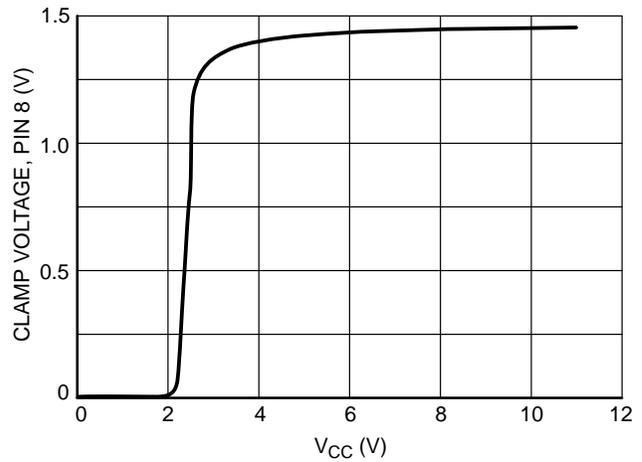
Figure 11. FB/SD Clamp Voltage versus V<sub>CC</sub>
