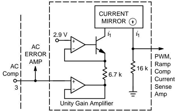
Figure 37. AC Reference Buffer Schematic
