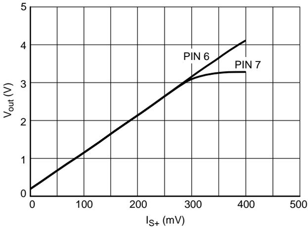
Figure 4. Current Sense Amplifier Gain
