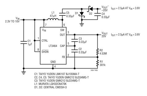
±20V Dual Output Converter with Output Disconnect
