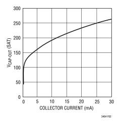
Figure 5: Output Disconnect Voltage Drop (V<sub>DROP</sub>) vs Current
