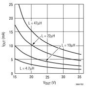
Figure 3. Maximum Output Current V<sub>IN</sub> = 8.4V
