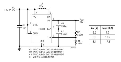
**15V Output Converter with Output Disconnect**
