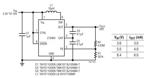
20V Output Converter with Output Disconnect Using an 0805 Inductor and 0603 Capacitors
