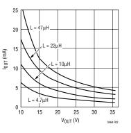
Figure 2. Maximum Output Current V<sub>IN</sub> = 5V
