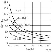
Figure 1. Maximum Output Current  $V_{IN} = 3.6V$
