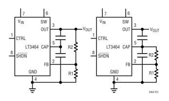
Figure 4. Feedback Connection Using the CAP Pin and the OUT Pin
