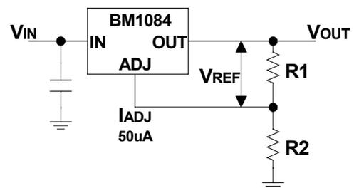
$$V_{OUT} = V_{REF} (1 + R2/R1) + I_{ADJ}R2$$
