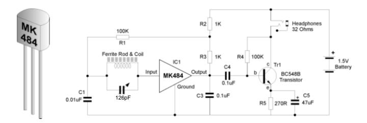
The coil needs approximately 55 turns of 0.315mm diameter enamelled copper wire on a 100mm long ferrite rod. A process of trial and error will help you achieve the optimum number of windings on the ferrite rod.
