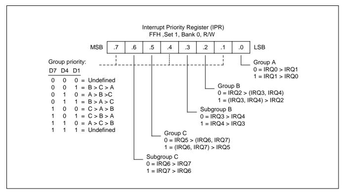
Figure 5-8. Interrupt Priority Register (IPR)
