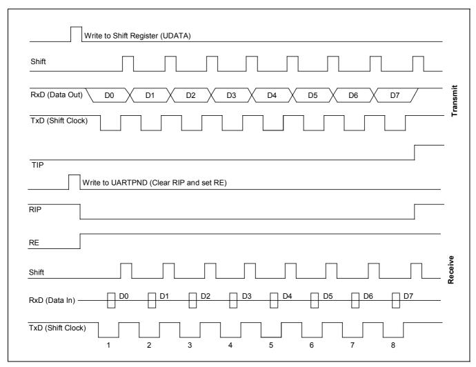
Figure 14-6. Timing Diagram for UART Mode 0 Operation
