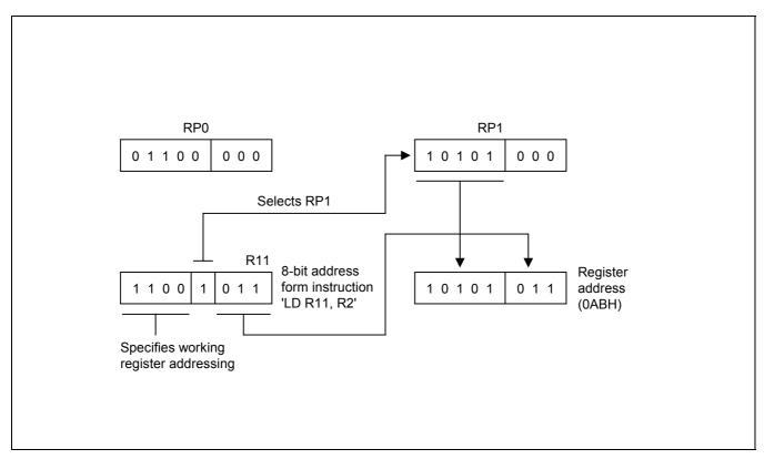
Figure 2-14. 8-Bit Working Register Addressing Example
