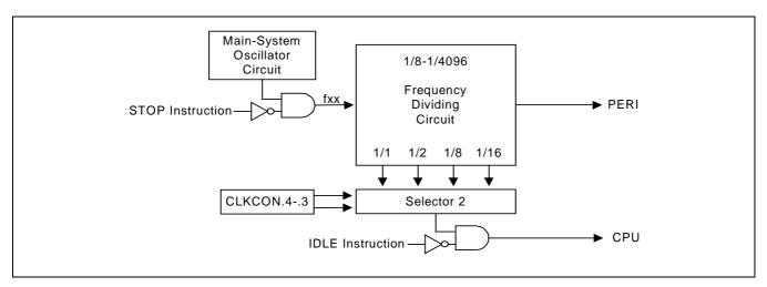
Figure 7-2. System Clock Circuit Diagram
