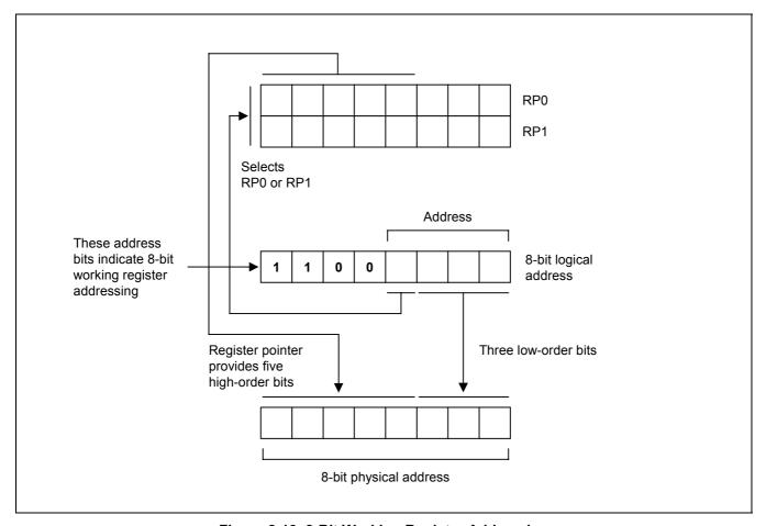
Figure 2-13. 8-Bit Working Register Addressing
