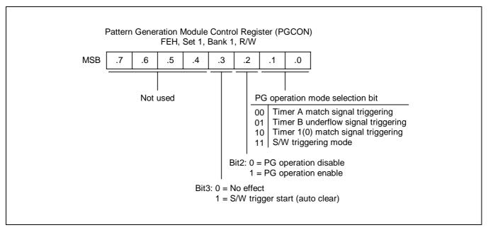
Figure 17-2. PG Control Register (PGCON)
