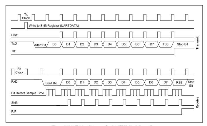
Figure 14-9. Timing Diagram for UART Mode 3 Operation
