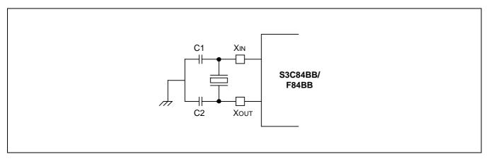
Figure 7-1. Main Oscillator Circuit (Crystal or Ceramic Oscillator)
