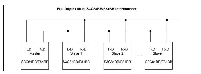
Figure 14-10. Connection Example for Multiprocessor Serial Data Communications
