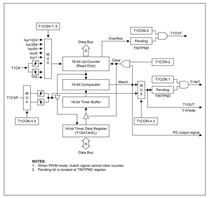
Figure 12-3. Timer 1(0/1) Functional Block Diagram
