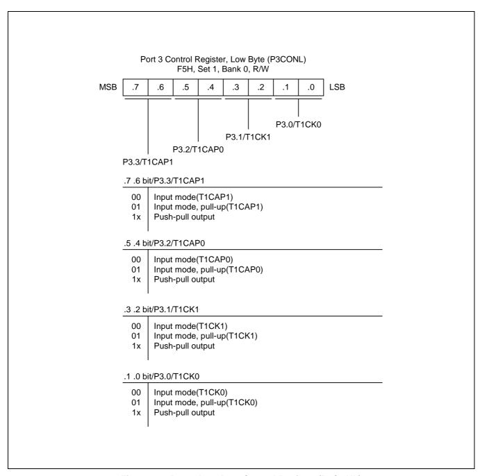
Figure 9-6. Port 3 Low-Byte Control Register (P3CONL)
