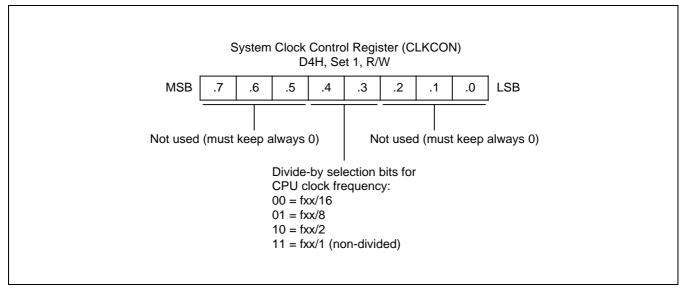
Figure 7-3. System Clock Control Register (CLKCON)
