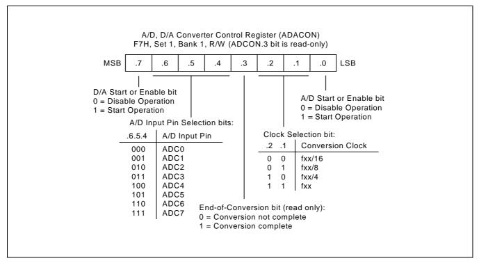
Figure 16-1. D/A Converter Control Register (ADACON)
