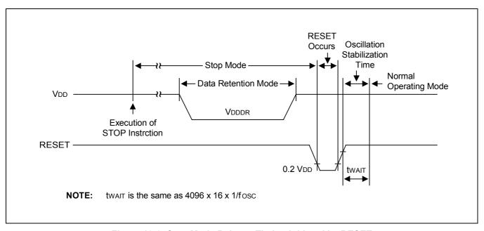
Figure 19-3. Stop Mode Release Timing Initiated by RESET
