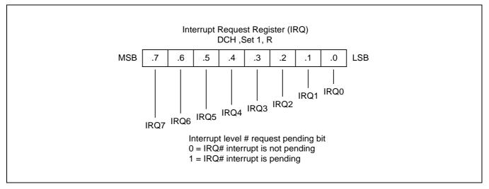
Figure 5-9. Interrupt Request Register (IRQ)
