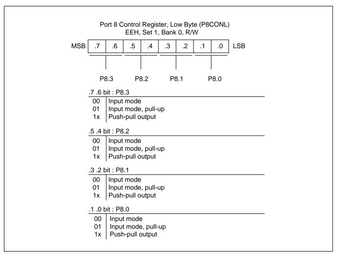
Figure 9-15. Port 8 Low-Byte Control Register (P8CONL)
