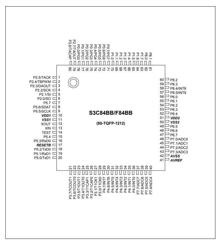
Figure 1-3. S3C84BB/F84BB Pin Assignment (80-TQFP)
