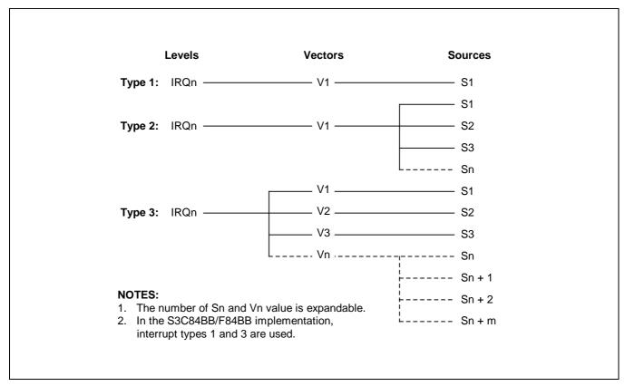
Figure 5-1. S3C8-Series Interrupt Types
