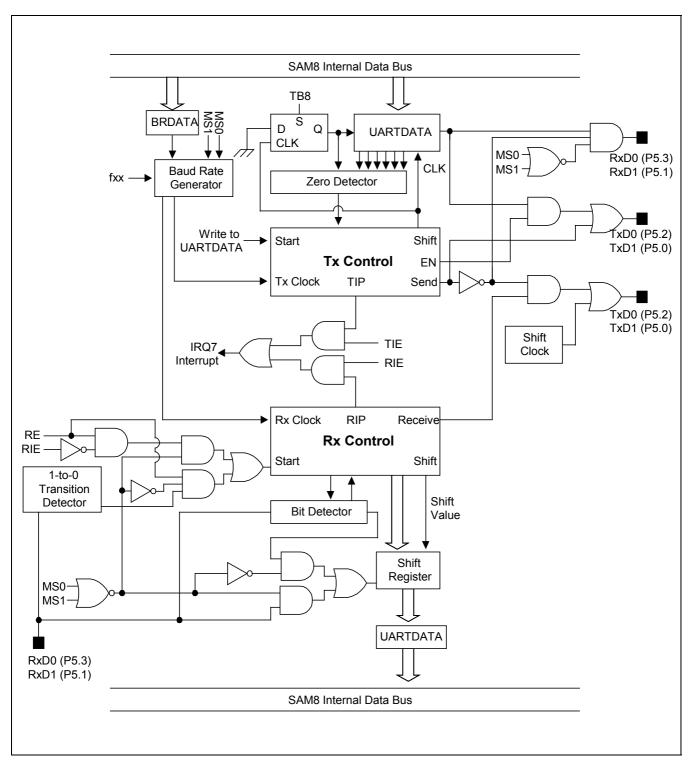
Figure 14-5. UART Functional Block Diagram
