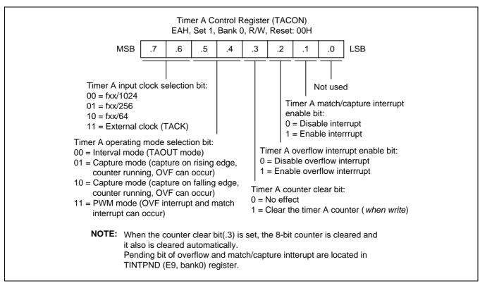
Figure 11-1. Timer A Control Register (TACON)
