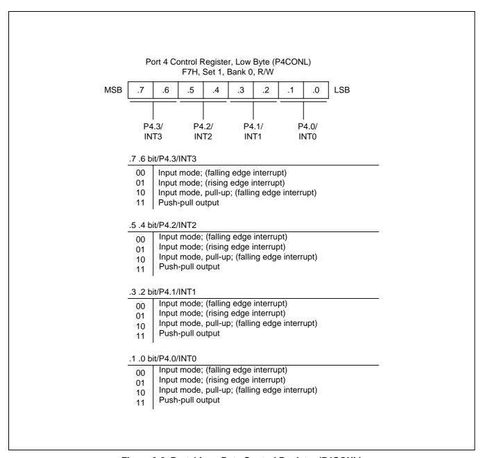
Figure 9-8. Port 4 Low-Byte Control Register (P4CONL)
