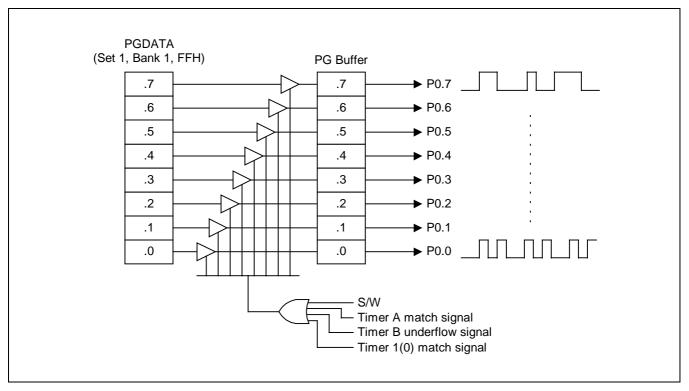
Figure 17-3. Pattern Generation Circuit Diagram
