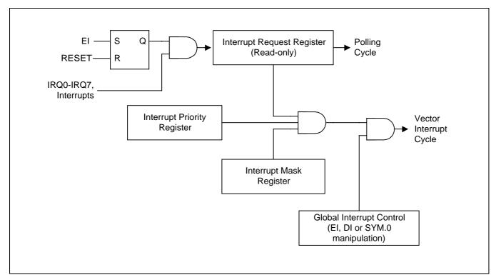
Figure 5-4. Interrupt Function Diagram
