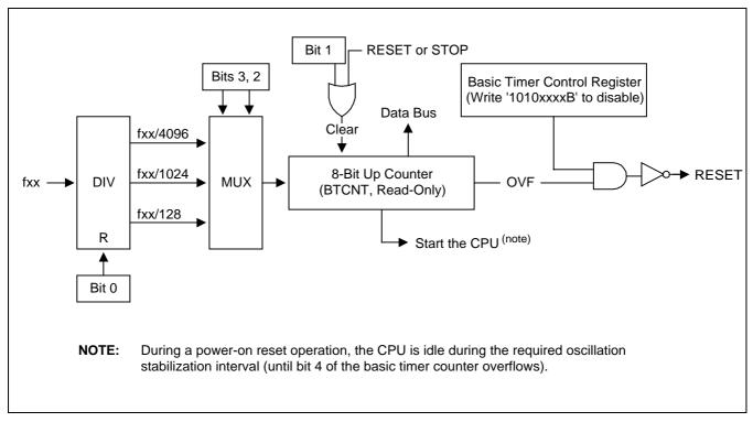
Figure 10-2. Basic Timer Block Diagram
