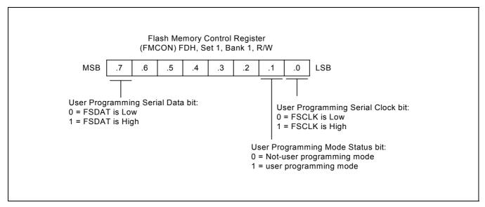
Figure 18-1. Flash Memory Control Register (FMCON)
