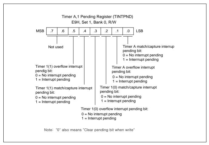
Figure 12-2. Timer A and Timer 1(0/1) Pending Register (TINTPND)
