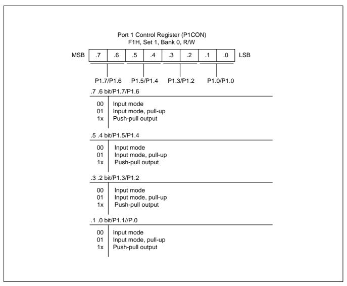
Figure 9-2. Port 1 Control Register (P1CON)
