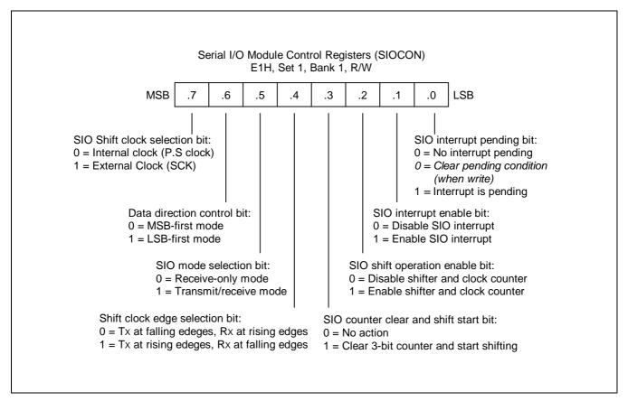
Figure 13-1. SIO Module Control Register (SIOCON)
