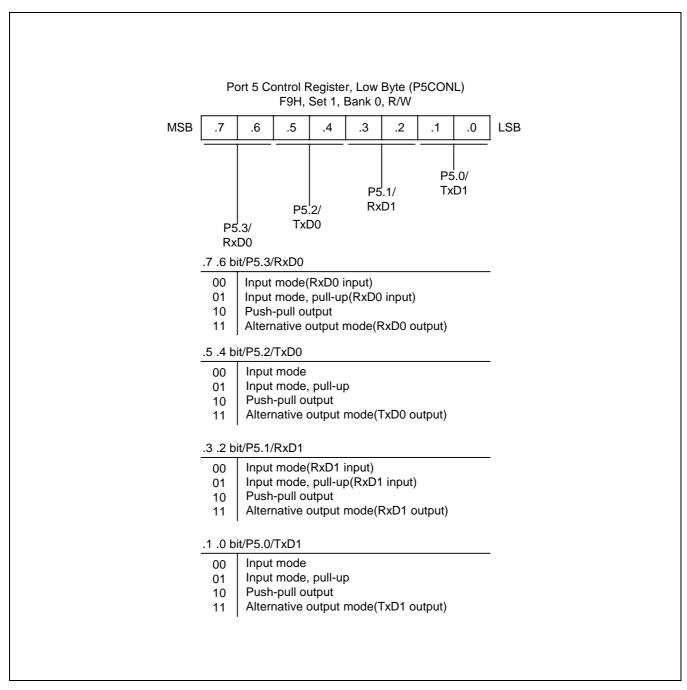
Figure 9-12. Port 5 Low-Byte Control Register (P5CONL)
