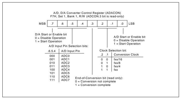
Figure 15-1. A/D Converter Control Register (ADACON)
