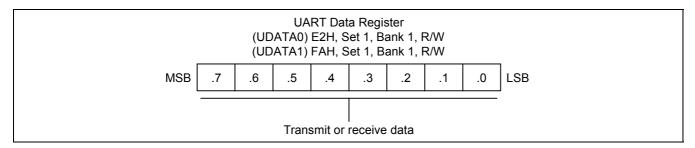
Figure 14-3. UART Data Register (UDATA0, UDATA1)
