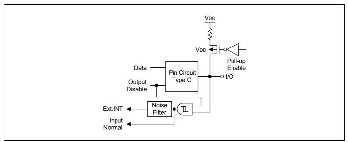
Figure 1-7. Pin Circuit Type D-1 (P4, P8.4, P8.5)
