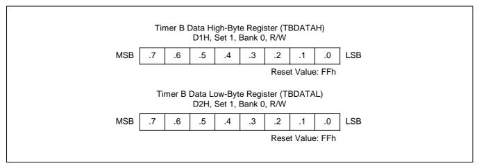
Figure 11-5. Timer B Data Registers (TBDATAH, TBDATAL)
