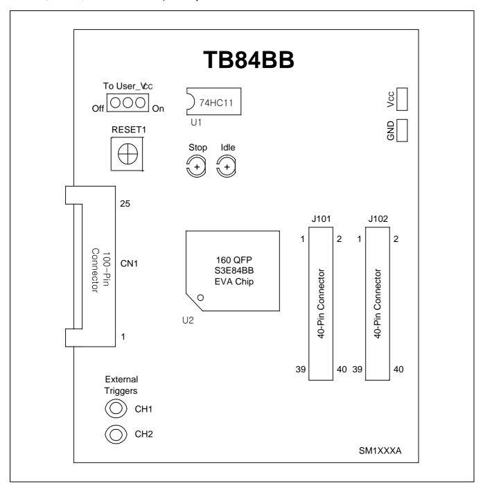
Figure 21–2. TB84BB Target Board Configuration
