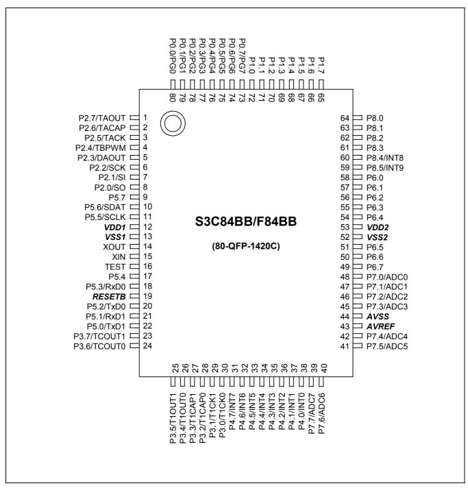
Figure 1-2. S3C84BB/F84BB Pin Assignment (80-QFP)
