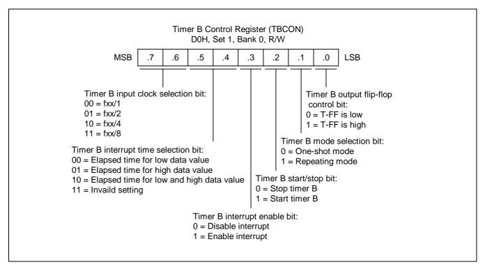
Figure 11-4. Timer B Control Register (TBCON)
