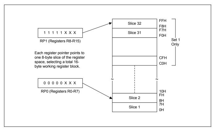
Figure 2-5. 8-Byte Working Register Areas (Slices)
