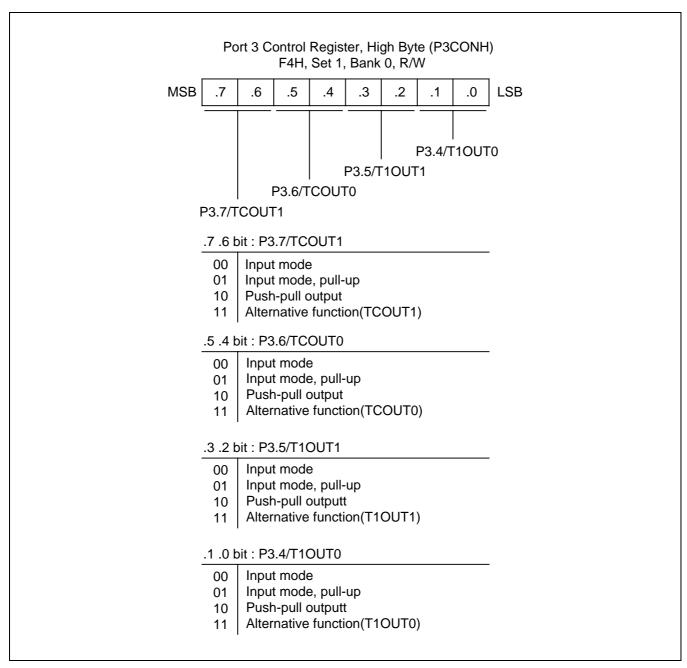
Figure 9-5. Port 3 High-Byte Control Register (P3CONH)
