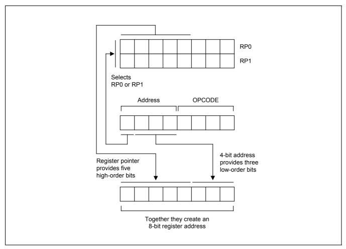
Figure 2-11. 4-Bit Working Register Addressing
