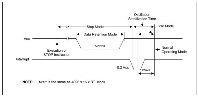
Figure 19-4. Stop Mode Release Timing Initiated by Interrupts
