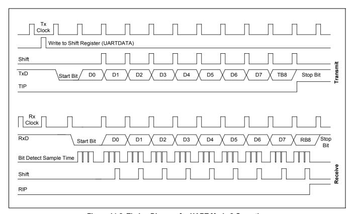
Figure 14-8. Timing Diagram for UART Mode 2 Operation
