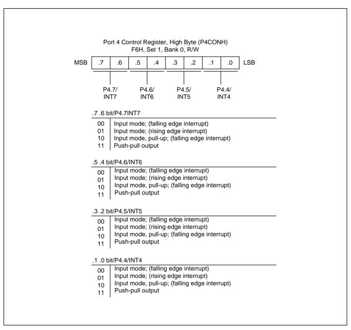
Figure 9-7. Port 4 High-Byte Control Register (P4CONH)
