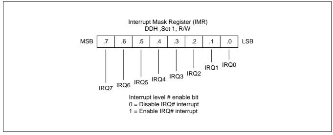
Figure 5-6. Interrupt Mask Register (IMR)
