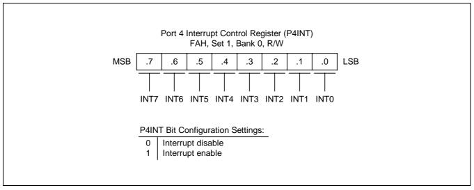
Figure 9-9. Port 4 Interrupt Control Register (P4INT)
