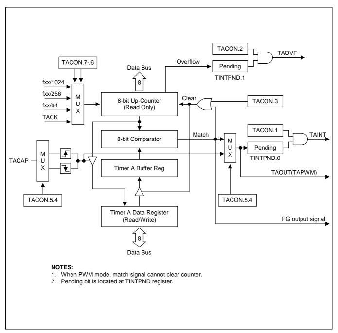
Figure 11-2. Timer A Functional Block Diagram
