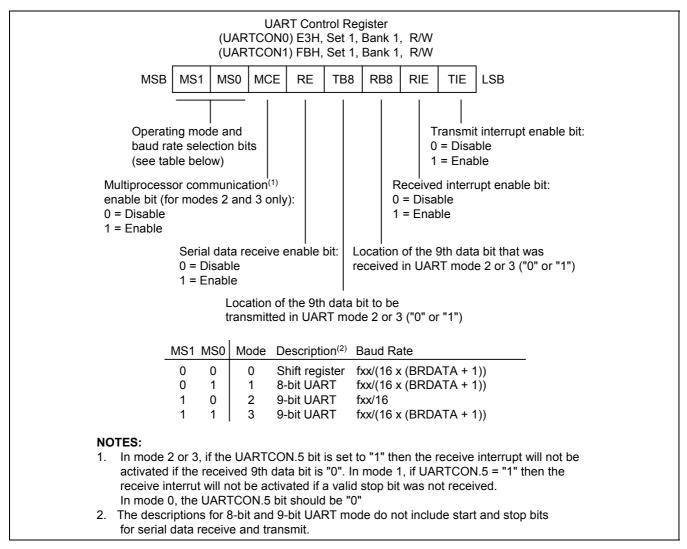
Figure 14-1. UART Control Register (UARTCON0, UARTCON1)
