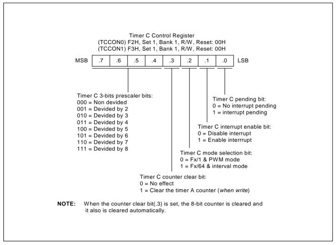
Figure 11-7. Timer C (0/1) Control Register (TCCON0, TCCON1)
