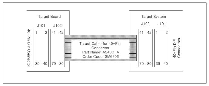
Figure 21-4. TB84BB Cable for 80-QFP Adapter
