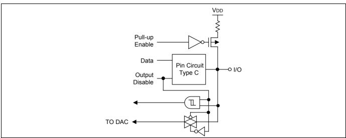
Figure 1-8. Pin Circuit Type D-2 (P2.3)
