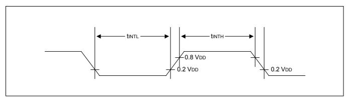
Figure 19-1. Input Timing for External Interrupts (Ports 4, Port 8.5, Port 8.6)
