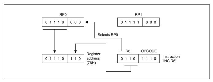
Figure 2-12. 4-Bit Working Register Addressing Example
