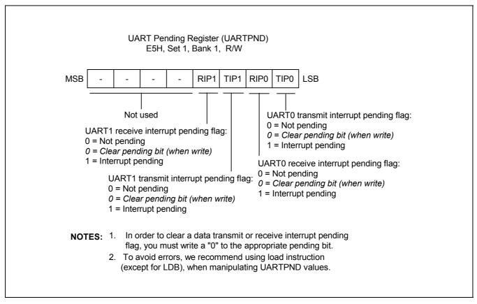
Figure 14-2. UART Interrupt Pending Register (UARTPND)
