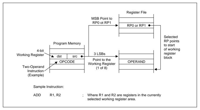
Figure 3-2. Working Register Addressing
