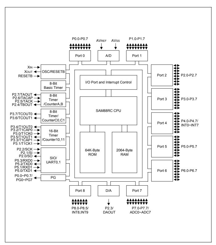
Figure 1-1. S3C84BB/F84BB Block Diagram
