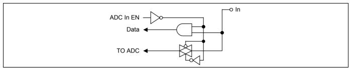
Figure 1-9. Pin Circuit Type E (ADC0-ADC7)
