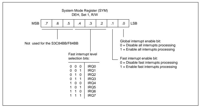
Figure 5-5. System Mode Register (SYM)
