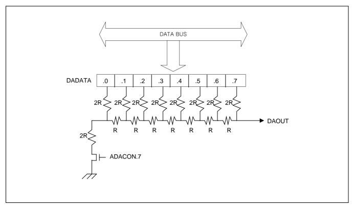
Figure 16-3. D/A Converter Circuit Diagram
