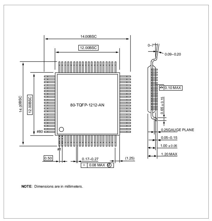
Figure 20–2. S3C84BB/F84BB 80-TQFP Standard Package Dimension (in Millimeters)
