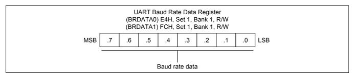
Figure 14-4. UART Baud Rate Data Register (BRDATA0, BRDATA1)
