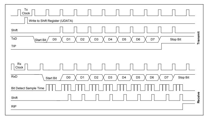
Figure 14-7. Timing Diagram for UART Mode 1 Operation
