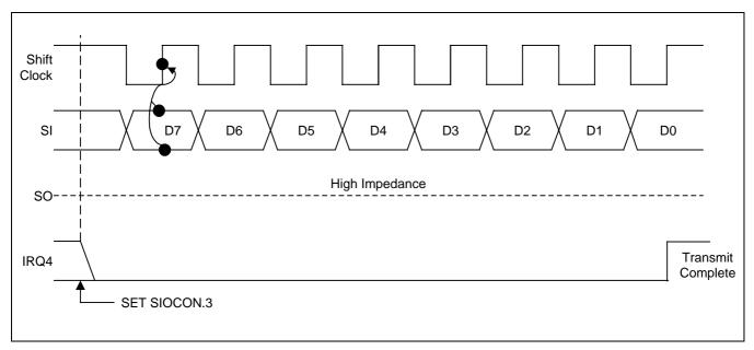
Figure 13-6. SIO Timing in Receive-Only Mode (Rising edge start)
