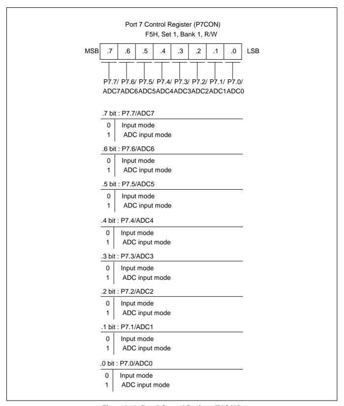
Figure 9-13. Port 7 Control Register (P7CON)
