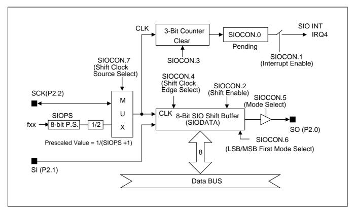
Figure 13-3. SIO Functional Block Diagram
