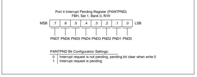
Figure 9-10. Port 4 Interrupt Pending Register (P4INTPND)
