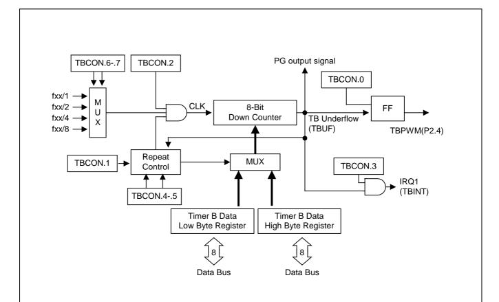
NOTE: In case of setting TBCON.5-.4 at '10', the value of the TBDATAL register is loaded into the 8-bit counter when the operation of the timer B starts. And then if a underflow occurs in the counter, the value of the TBDATAH register is loaded with the value of the 8-bit counter. However, if the next borrow occurs, the value of the TBDATAL register is loaded with the value of the 8-bit counter. To output TBPWM as carrier wave, you have to set P2CONH.1-.0 as "11".
