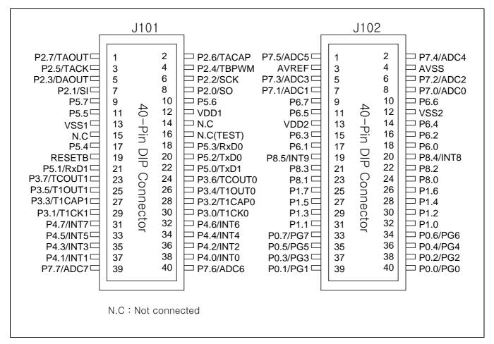
Figure 21–3. 40-Pin Connectors for TB84BB (S3C84BB, 80-QFP Package)
