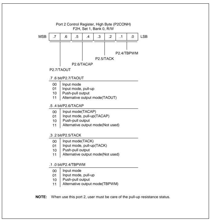
Figure 9-3. Port 2 High-Byte Control Register (P2CONH)
