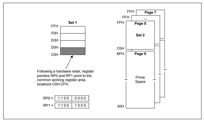
Figure 2-10. Common Working Register Area
