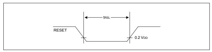
Figure 19-2. Input Timing for RESET
