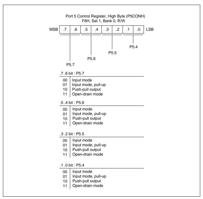
Figure 9-11. Port 5 High-Byte Control Register (P5CONH)
