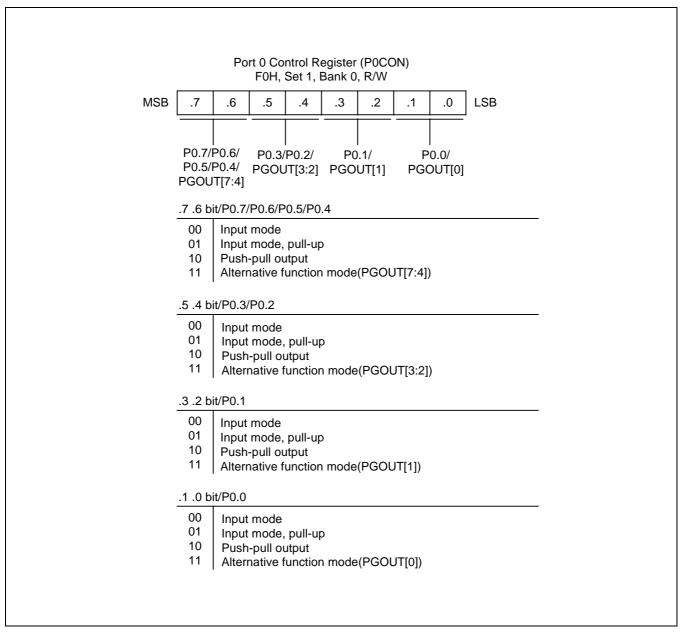
Figure 9-1. Port 0 Control Register (P0CON)
