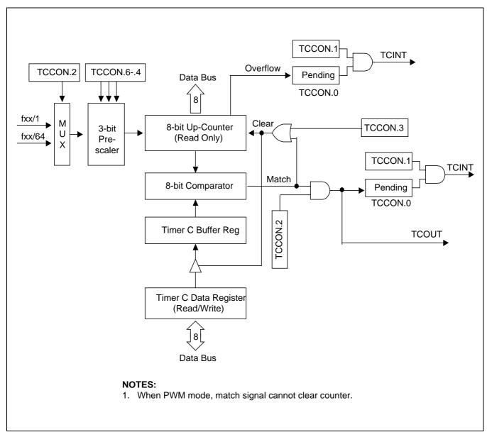
Figure 11-8. Timer C (0/1) Functional Block Diagram
