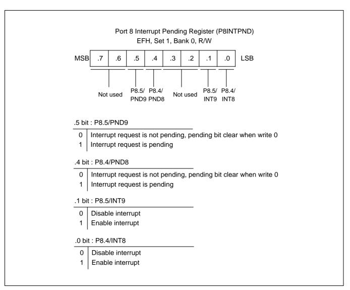
Figure 9-16. Port 8 Interrupt Pending Register (P8INTPND)
