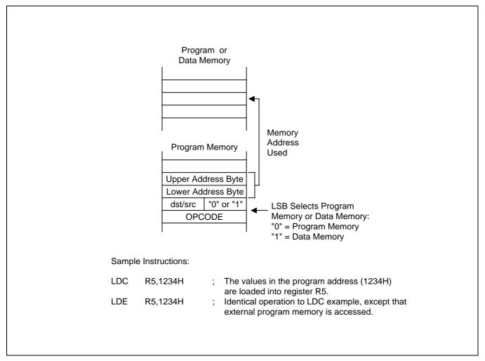
Figure 3-10. Direct Addressing for Load Instructions
