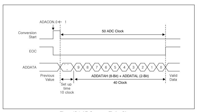
Figure 15-4. A/D Converter Timing Diagram
