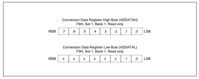
Figure 15-2. A/D Converter Data Register (ADDATAH, ADDATAL)
