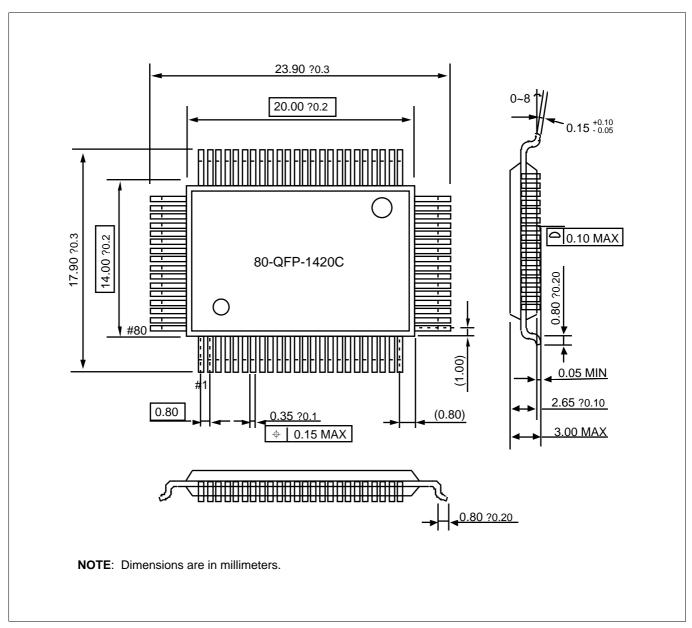
Figure 20–1. S3C84BB/F84BB 80-QFP Standard Package Dimension (in Millimeters)
