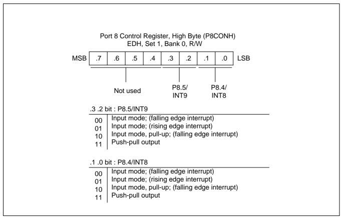
Figure 9-14. Port 8 High-Byte Control Register (P8CONH)
