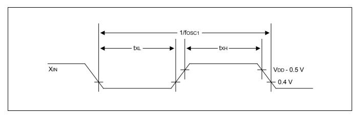
Figure 19-5. Clock Timing Measurement at  $\mathbf{X}_{\text{IN}}$
