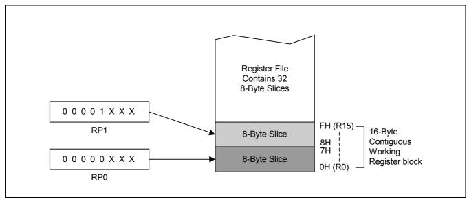
Figure 2-6. Contiguous 16-Byte Working Register Block
