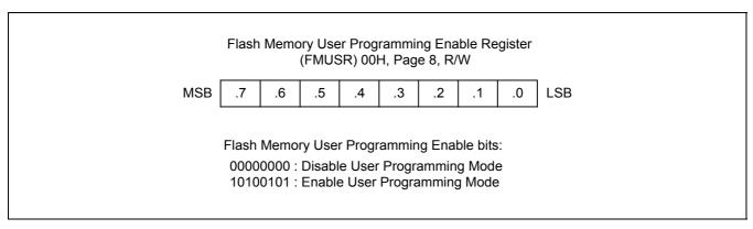
Figure 18-2. Flash Memory User Programming Enable Register (FMUSR)
