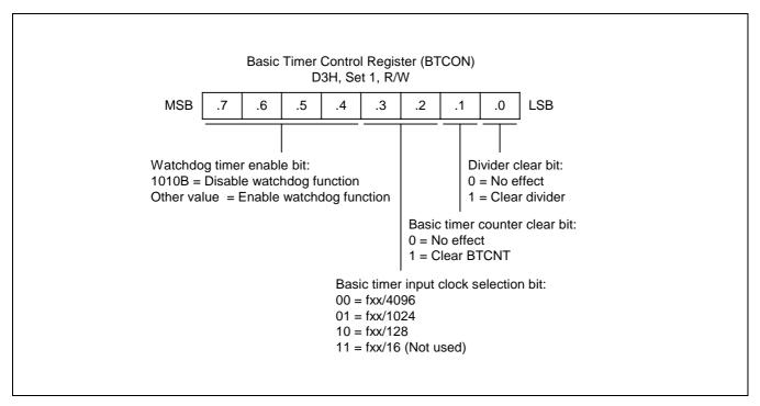
Figure 10-1. Basic Timer Control Register (BTCON)
