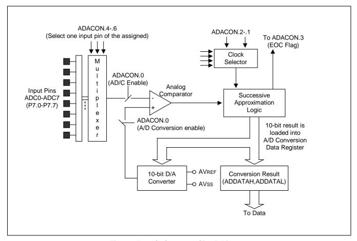
Figure 15-3. A/D Converter Circuit Diagram
