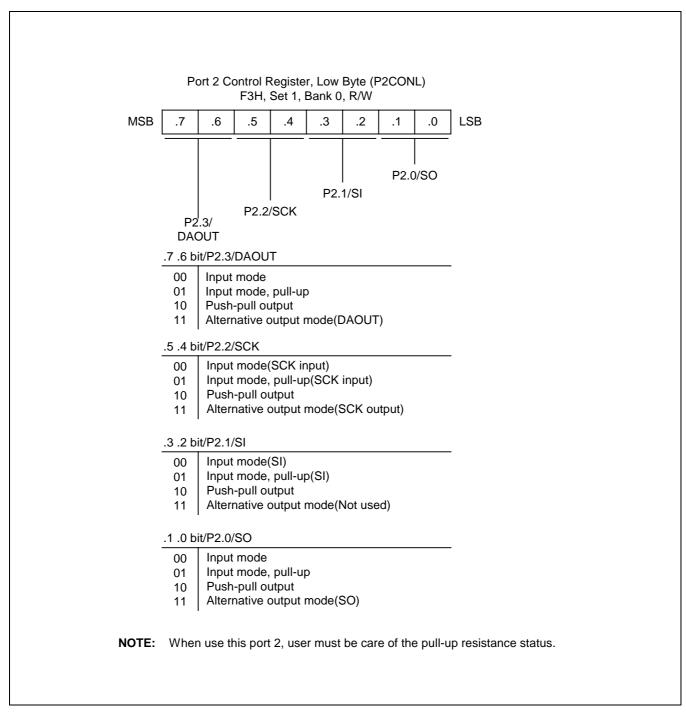
Figure 9-4. Port 2 Low-Byte Control Register (P2CONL)
