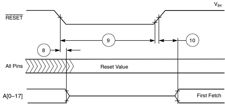
Figure 2-3. Reset Timing
