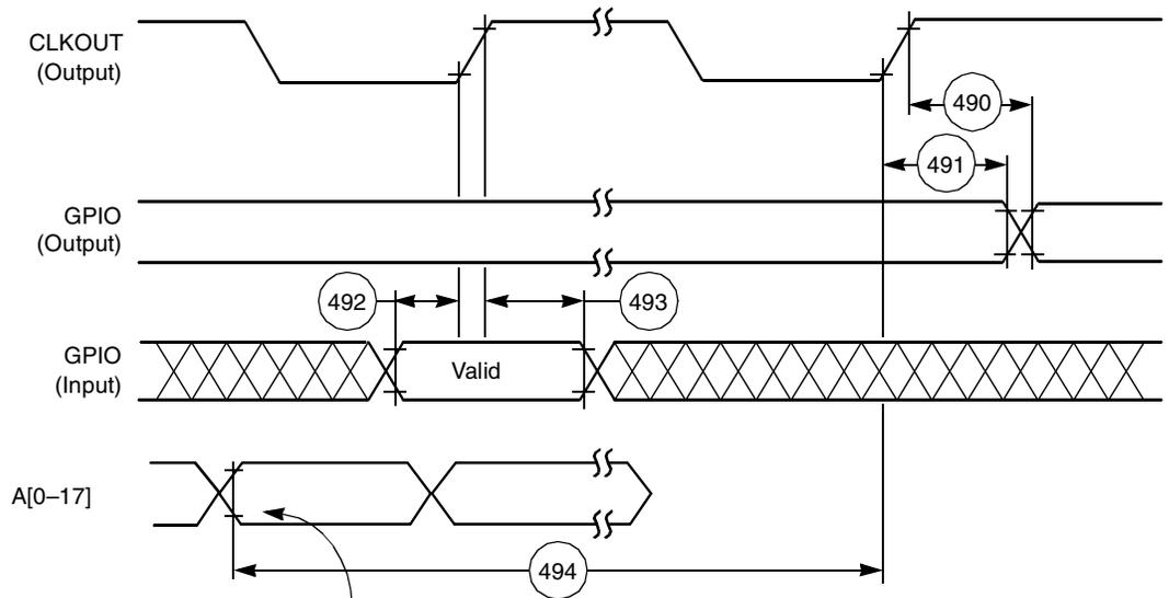
Fetch the instruction MOVE X0,X:(R0); X0 contains the new value of GPIO and R0 contains the address of the GPIO data register.
