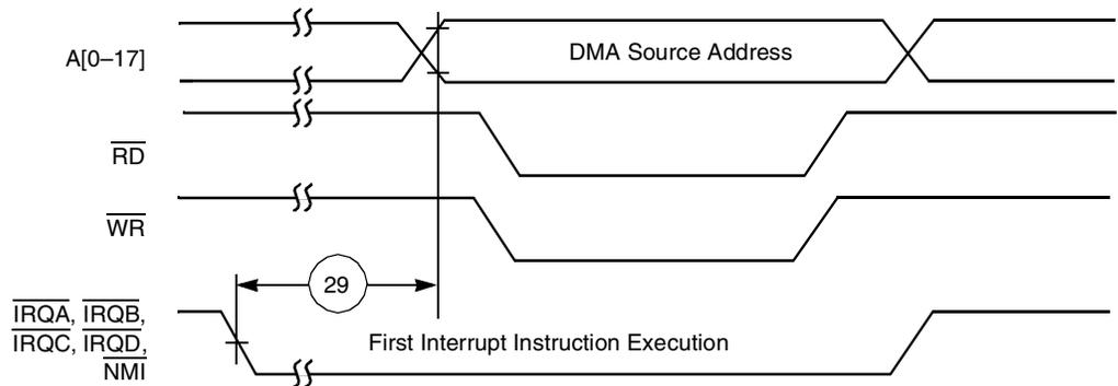
Figure 2-9. External Memory Access (DMA Source) Timing
