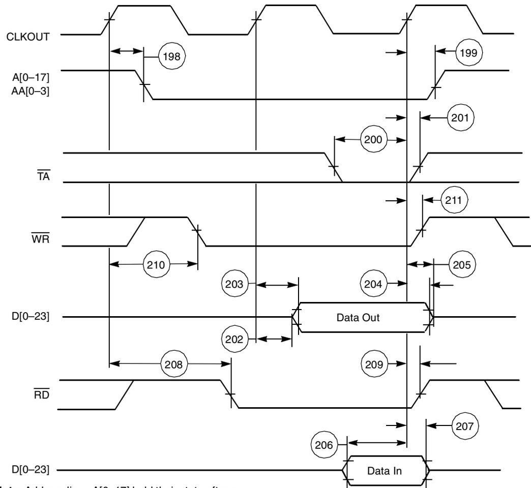
**Note:** Address lines A[0-17] hold their state after a read or write operation. AA[0-3] do not hold their state after a read or write operation.
