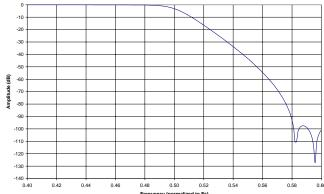
Figure 33. Single Speed Mode Stopband Rejection
