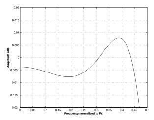
Figure 48. Single Speed (fast) Passband Ripple
