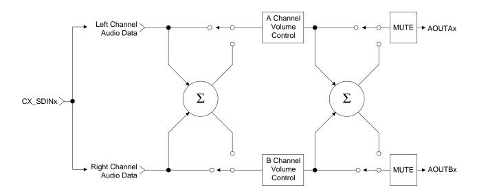
Figure 8. ATAPI Block Diagram (x = channel pair 1, 2, 3, 4)
