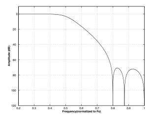
Figure 57. Double Speed (slow) Stopband Rejection
