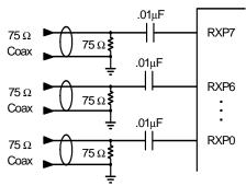
Figure 31. S/PDIF MUX Input Circuit
