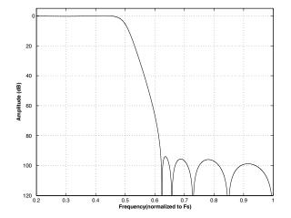
Figure 61. Quad Speed (fast) Stopband Rejection
