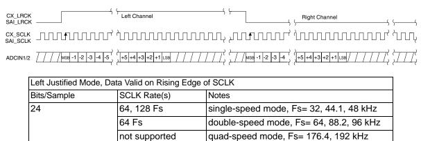
Figure 15. ADCIN1/ADCIN2 Serial Audio Format
