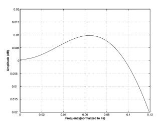
Figure 68. Quad Speed (slow) Passband Ripple
