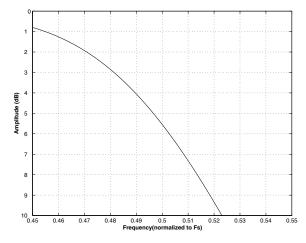
Figure 67. Quad Speed (slow) Transition Band (detail)
