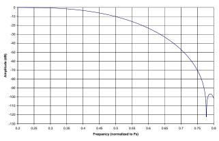
Figure 41. Quad Speed Mode Stopband Rejection
