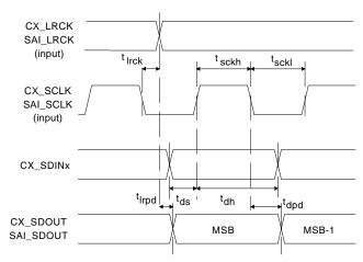
Figure 2. Serial Audio Port Slave Mode Timing
