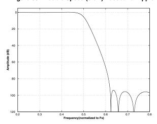
Figure 62. Quad Speed (fast) Transition Band
