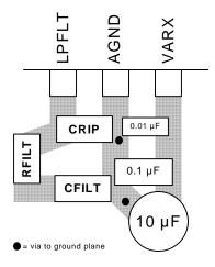
Figure 29. Recommended Layout Example
