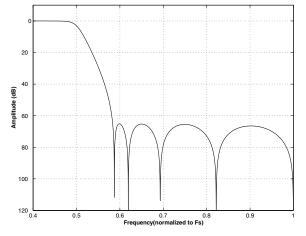
Figure 49. Single Speed (slow) Stopband Rejection
