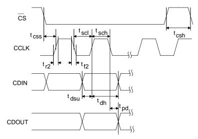
Figure 4. Control Port Timing - SPI Format
