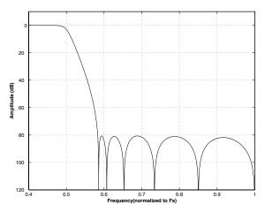
Figure 53. Double Speed (fast) Stopband Rejection
