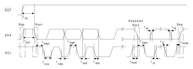
Figure 3. Control Port Timing - I<sup>2</sup>C Format
