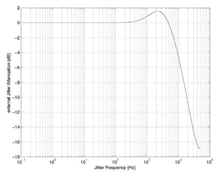
Figure 28. Jitter Attenuation Characteristics of PLL
