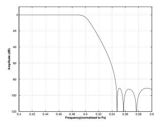
Figure 46. Single Speed (fast) Transition Band
