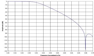
Figure 37. Double Speed Mode Stopband Rejection
