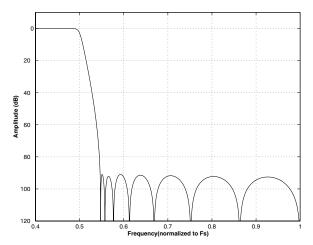
Figure 45. Single Speed (fast) Stopband Rejection
