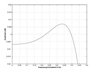
Figure 52. Single Speed (slow) Passband Ripple
