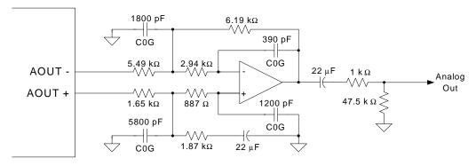
Figure 25. Recommended Analog Output Buffer
