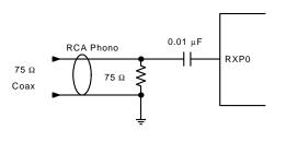
Figure 30. Consumer Input Circuit
