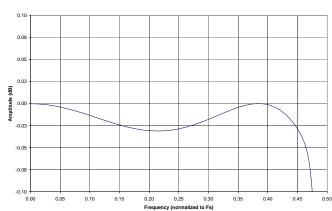
Figure 35. Single Speed Mode Transition Band (Detail)
