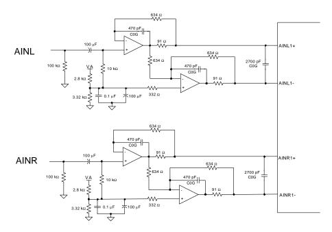
Figure 24. Recommended Analog Input Buffer
