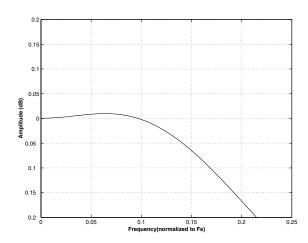
Figure 64. Quad Speed (fast) Passband Ripple
