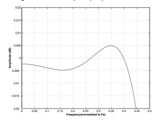
Figure 56. Double Speed (fast) Passband Ripple
