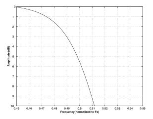
Figure 63. Quad Speed (fast) Transition Band (detail)
