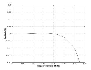
Figure 60. Double Speed (slow) Passband Ripple
