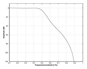
Figure 65. Quad Speed (slow) Stopband Rejection
