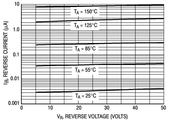
Figure 3. Leakage Current
