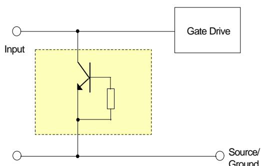
Input is not designed for DC current > 2 mA
