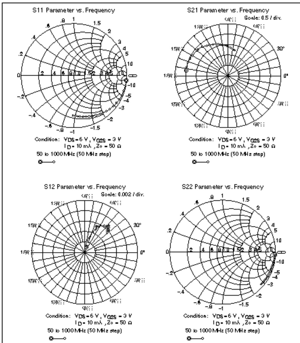
**S Parameter** ( $V_{DS} = 6\text{ V}$ ,  $V_{G2S} = 3\text{ V}$ ,  $I_D = 10\text{ mA}$ ,  $Z_0 = 50\ \Omega$ )
