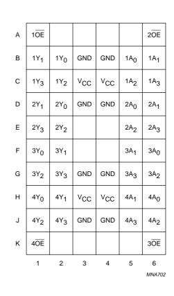
Fig.2 Pin configuration VFBGA56.
