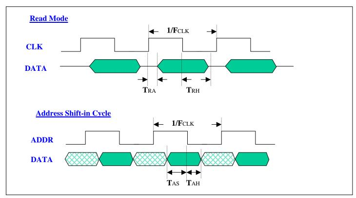
Note: The duty cycle of any clock is 50%
