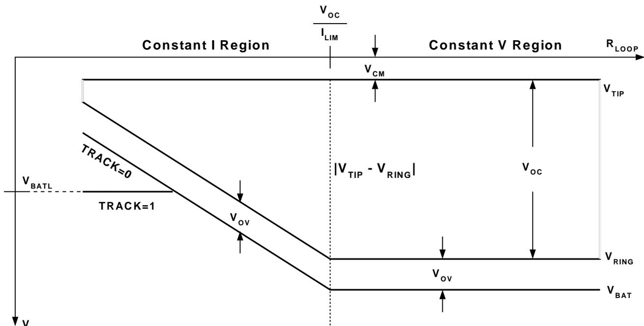
Figure 15.  $V_{TIP}$ ,  $V_{RING}$ , and  $V_{BAT}$  in the Forward Active State
