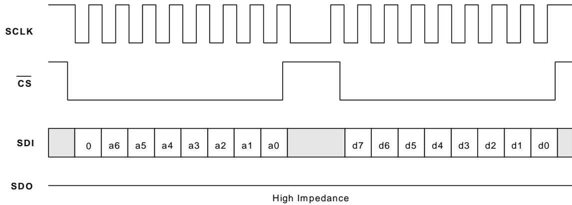
**Figure 23. Serial Write 8-Bit Mode**
