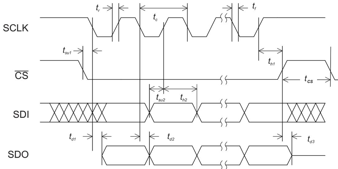
**Figure 7. SPI Interface Timing Diagram**
