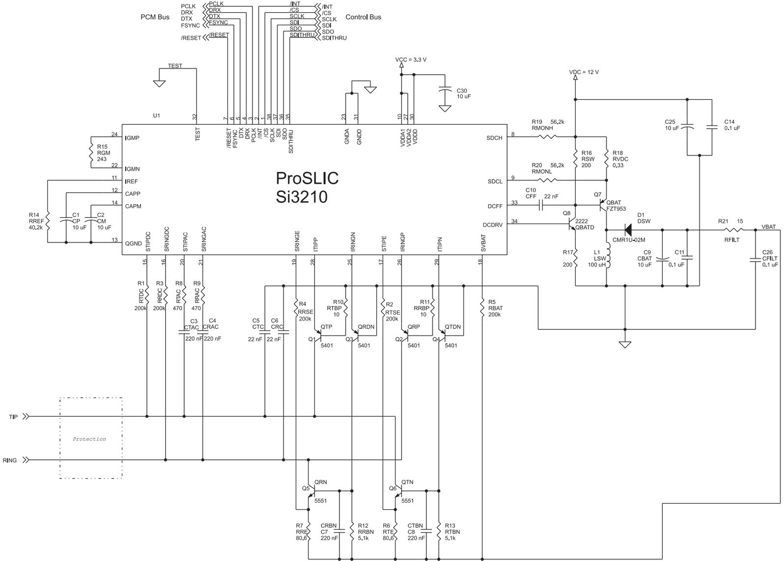
Figure 9. Si3210 Typical Application Circuit Using DC-to-DC Converter
