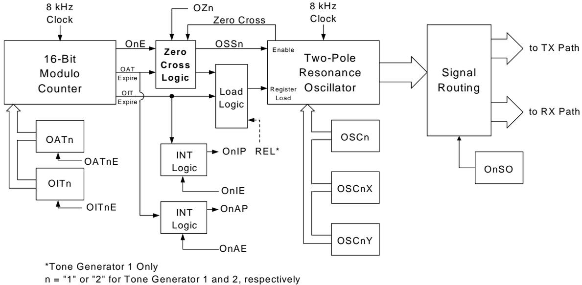
**Figure 17. Simplified Tone Generator Diagram**
