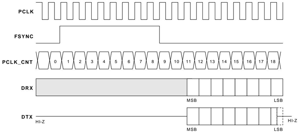
**Figure 28. Example, IDL2 Long FSYNC, B2, 10-Bit Mode (TXS/RXS = 10)**
