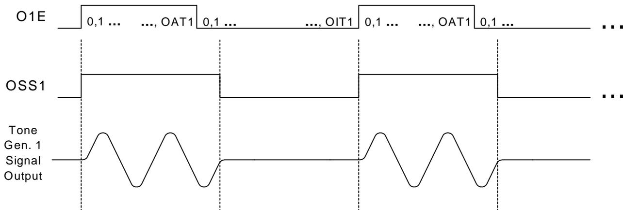
**Figure 18. Tone Generator Timing Diagram**
