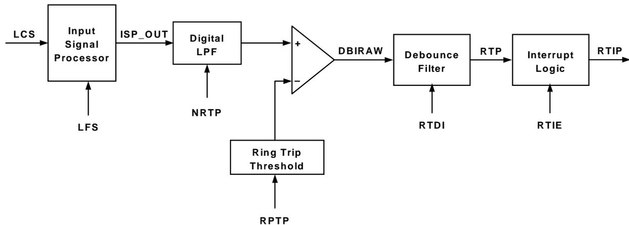
Figure 20. Ring Trip Detector
