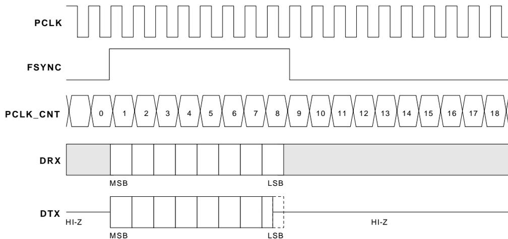
**Figure 27. Example, Timeslot 1, Long FSYNC (TXS/RXS = 0)**
