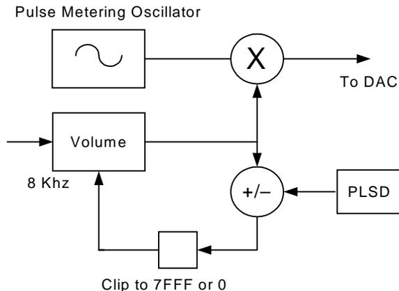
Figure 21. Pulse Metering Volume Envelope
