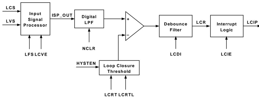
Figure 13. Loop Closure Detection
