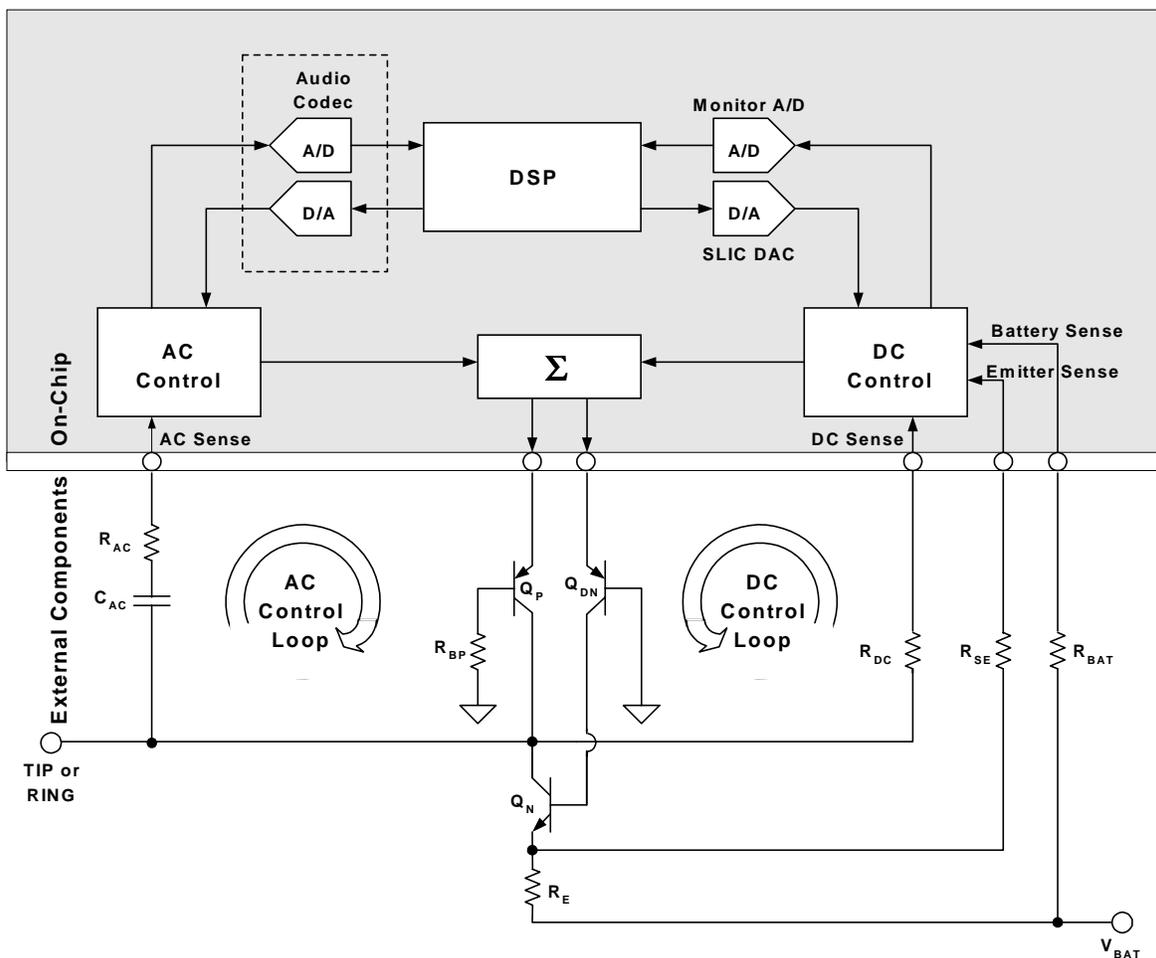
Figure 12. Simplified ProSLIC Linefeed Architecture for TIP and RING Leads (One Shown)
