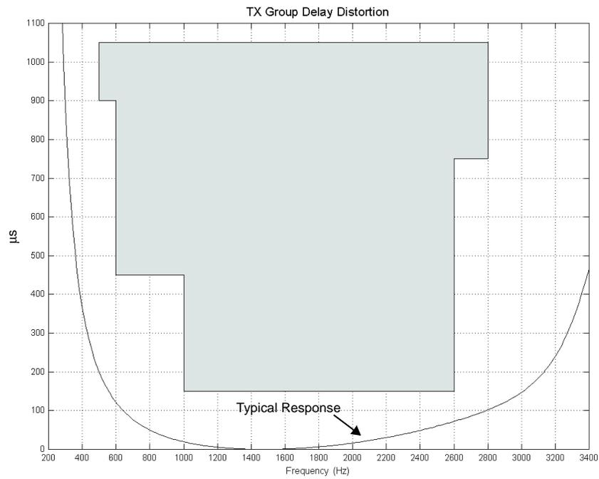
Figure 5. Transmit Group Delay Distortion
