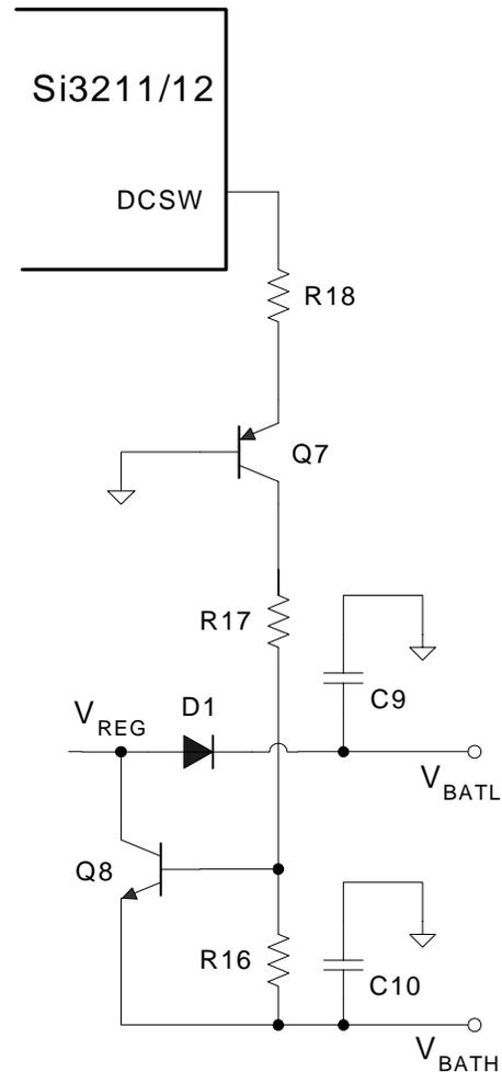
**Figure 16. Circuit Solution for Battery Switching**
