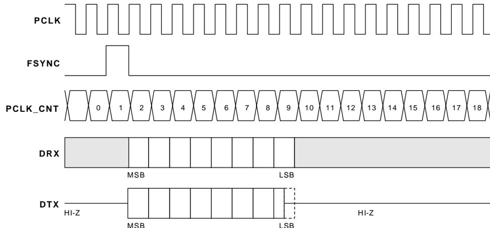
**Figure 26. Example, Timeslot 1, Short FSYNC (TXS/RXS = 1)**
