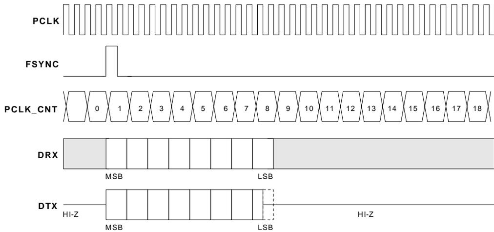
**Figure 29. GCI Example, Timeslot 1 (TXS/RXS = 0)**
