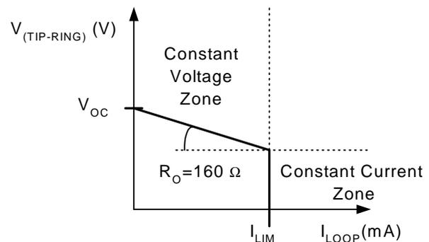
**Figure 11. Simplified DC Current/Voltage Linefeed Characteristic**
