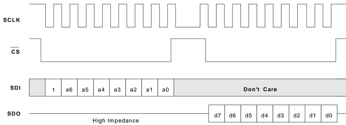
**Figure 24. Serial Read 8-Bit Mode**
