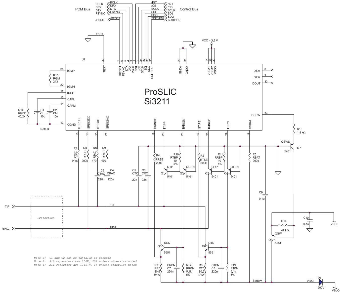
Figure 10. Si3210/11/12 Typical Application Circuit Using External Battery
