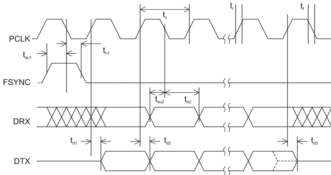
Figure 8. PCM Highway Interface Timing Diagram
