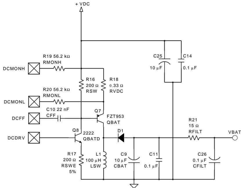
Figure 14. Typical DC-to-DC Converter Application Circuit
