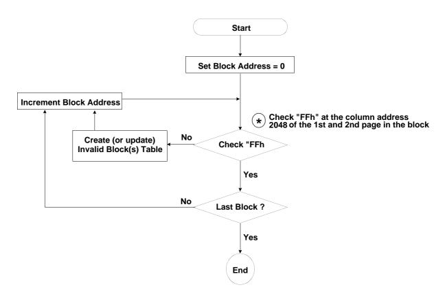
Figure 3. Flow chart to create invalid block table.
