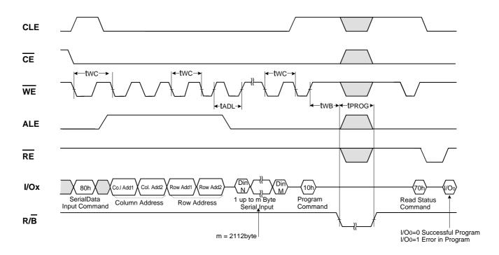
**NOTES:** tADL is the time from the  $\overline{\text{WE}}$  rising edge of final address cycle to the  $\overline{\text{WE}}$  rising edge of first data cycle.
