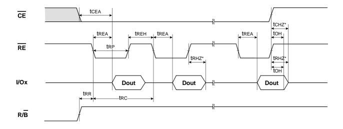
NOTES: Transition is measured  $\pm 200 \text{mV}$  from steady state voltage with load. This parameter is sampled and not 100% tested.
