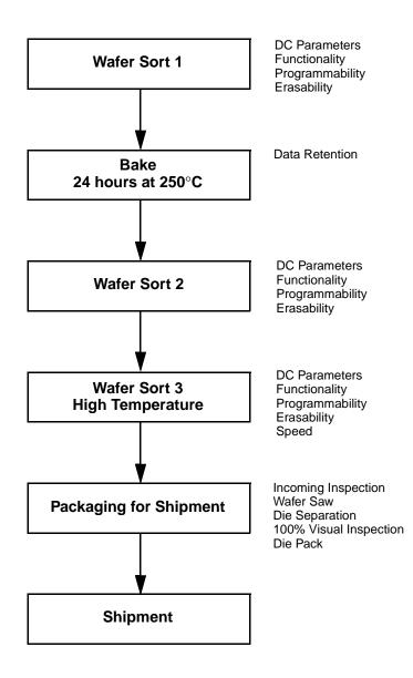
Figure 1. AMD KGD Product Test Flow
