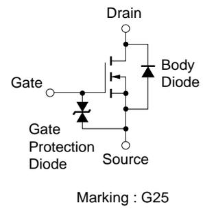
**Remark** The diode connected between the gate and source of the transistor serves as a protector against ESD. When this device actually used, an additional protection circuit is externally required if a voltage exceeding the rated voltage may be applied to this device.
