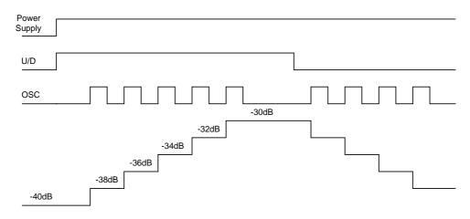
When the UP key is pressed after power ON, the U/D terminal is place in the UP state at "H" level, and the oscillator is actuated. When the DOWN key is pressed, the U/D terminal is kept at "L" level as long as the Down key is pressed, and the oscillator is actuated in the down state and therefore, attenuation is decreased. Oscillation frequency is decided by Cx and Rx.
