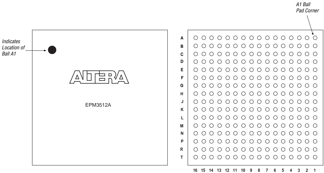
Figure 18. 256-Pin FineLine BGA Package Pin-Out Diagram
