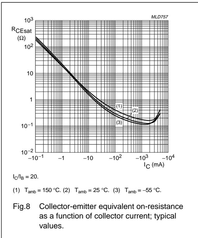
50 V low  $V_{CEsat}$  PNP transistor
