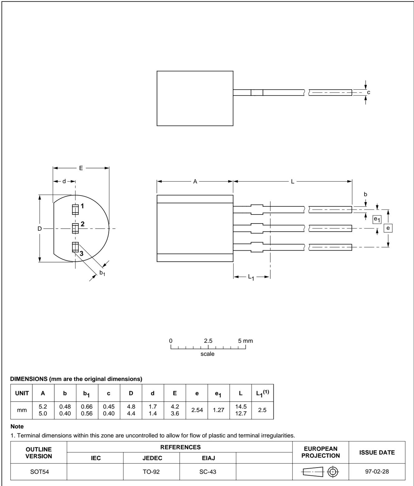
50 V low  $V_{CEsat}$  PNP transistor
