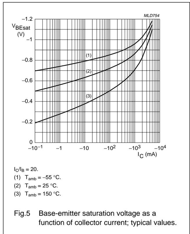
50 V low  $V_{CEsat}$  PNP transistor
