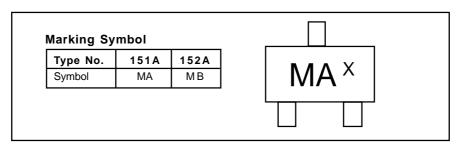
The "X" represents a smaller alpha digit Date Code. The Date Code indicates the actual month in which the part was manufactured.
