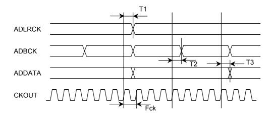
The figure above applies when the 48-bit slot is used for the audio data output slot.
