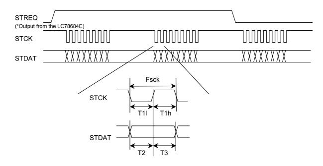
Performing a serial data input operation requires that a serial input command be issued.
