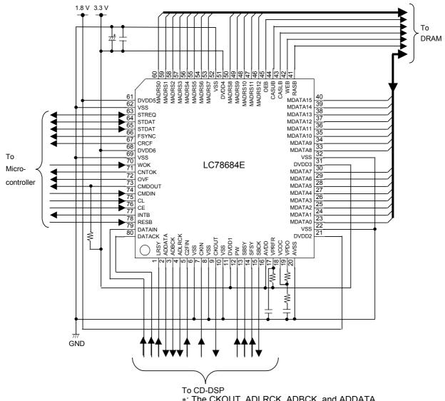
\*: The CKOUT, ADLRCK, ADBCK, and ADDATA pins must be connected to a CD DSP that supports external D/A converter input.
