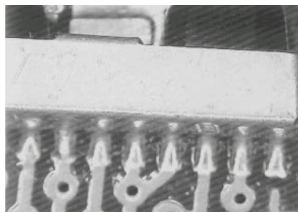
Photo 4.0. Unit self-aligns after reflow.
