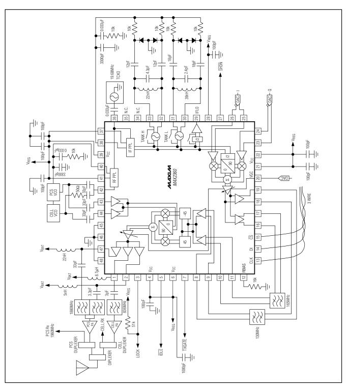
Figure 2. MAX2360 Typical Application Circuit
