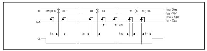
Figure 5. 3-Wire Interface Diagram
