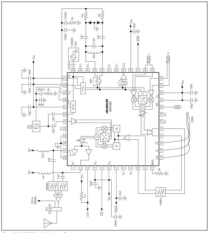
Figure 3. MAX2362 Typical Application Circuit
