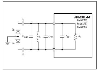
Figure 6. Tank Port Oscillator
