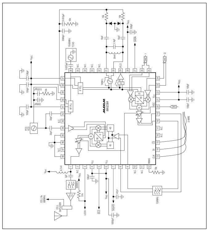
Figure 4. MAX2364 Typical Application Circuit
