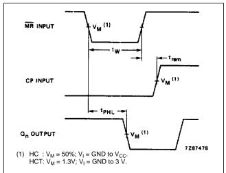
Fig.7 Waveforms showing the master reset  $(\overline{MR})$  pulse width, the master reset to output  $(Q_n)$  propagation delays and the master reset to clock (CP) removal time
