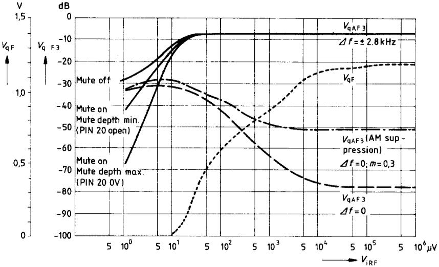
**Mixer Output Voltage  $V_{qIF}$  with Reference to 775 mV<sub>rms</sub> at 18 k $\Omega$  versus Input Level  $P_{iRF}$**
