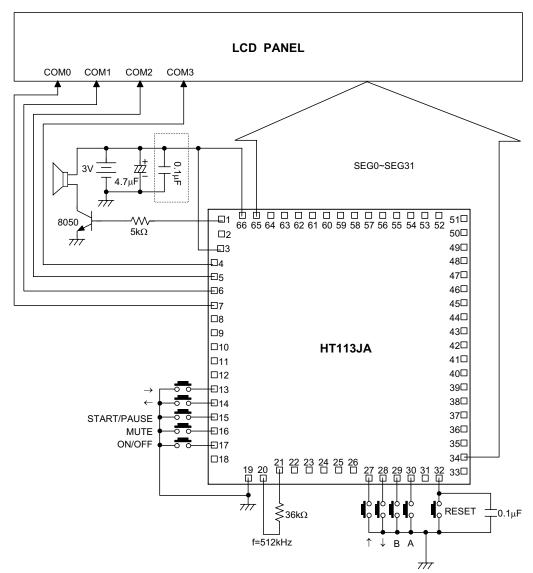
Note: The capacitor in dash block is recommended.
