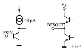
All information about reception conditions is derived from the fieldstrength voltage. The fieldstrength voltage at FSIN is initially buffered so as not to impair the characteristics of the IF IC and is available at BFSOUT. AVFS
