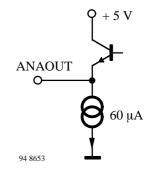
Analyzer output. DC values are available at this pin that characterize the respective reception situation. The output voltage is limited to max. 5 V. ANAOUT is a multiplex output, i.e. the value for the fieldstrength, level of multipath interference or level of common channel interference is applied to this output depending on addressing. ANAOUT can be switched to the high-impedance state by means of OE.
