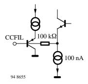
The controller element detects the absolute value of occuring common channel interference. This information is stored in a capacitor which must be connected externally to CGFIL. The capacitor voltage can be selected by the system controller and then available via ANAOUT.
