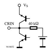
The internal one-pin oscillator is connected to CRIN with a 456 kHz ceramic resonator. The 456 kHz reference frequency is used for calibrating the filters and generating pulses at INT.
