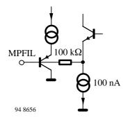
The controller element detects the absolute value of occuring multipath interference. This information is stored in a capacitor which must be connected externally to MPFIL. The capacitor voltage can be interrogated by the system controller via ANAOUT.
