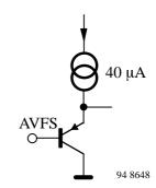
The fieldstrength signal at buffer output BFSOUT is averaged over time and applied to input AVFS via an RC low-pass filter with a large time constant.
