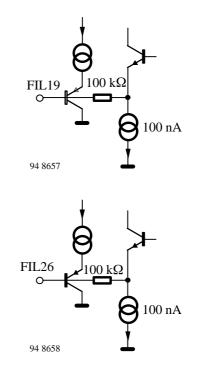
In order to differentiate the various types of interference, the amplitudes of a few spectral components of the fieldstrength signal are determined and filtered in FIL19 and FIL26 for further processing.
