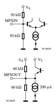
The MPX signal is fed directly from the FM demodulator to input MPXIN and is available amplified by a factor of 1.5 at MPXOUT. The MPX signal is blanked out in the event of multipath interference or when MUTE is activated externally in the circuit part MNC (Multipath Noise Canceller). In all other cases, the MPX signal passes through the IC unchanged.
