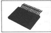
Thick Film Hybrid Integrated Circuit
