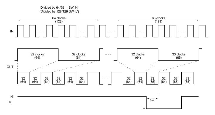
tset = The minimum time required between 'Modulus Control' going low and next output rising edge, in order to ensure a P+1 modulus change.
