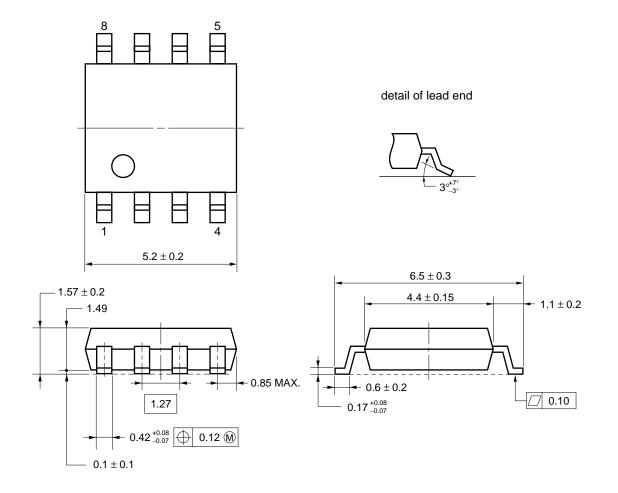
NOTE Each lead centerline is located within 0.12 mm of its true position (T.P.) at maximum material condition.
