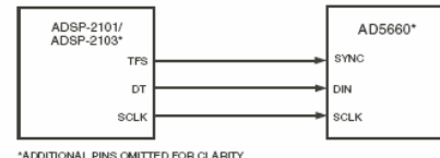
Figure 26. AD5660 to ADSP-2101/ADSP-2103 Interface
