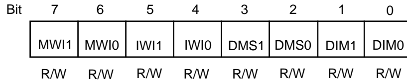
Figure 74. DMA/WAIT Control Register (DCNTL: I/O Address = 32H)
